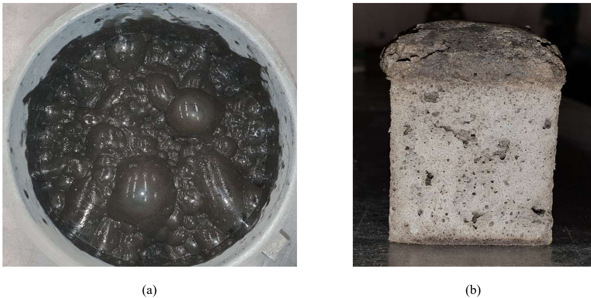
Figure 4 - \text{H}_2 gas formation in the preparation of mortars (a) and expanded mortar (b)
