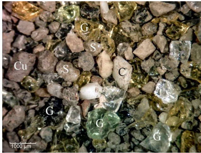
Figure 2 - Stereomicroscopic image of a sample of washed MIBA (G - glass with different colours; C - different kinds of ceramic; S - siliceous sand particles; Cu - copper-based metallic agglomerate, also containing iron and aluminium)
