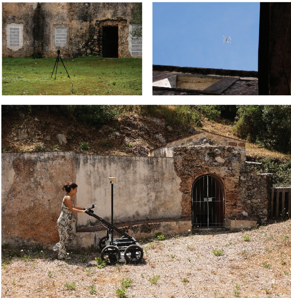
Figure 2. Digital surveying at the Capuchos Convent. Top left: TLS survey; top right: UAV photogrammetry. Bottom: GPR survey of the cooling house area.
