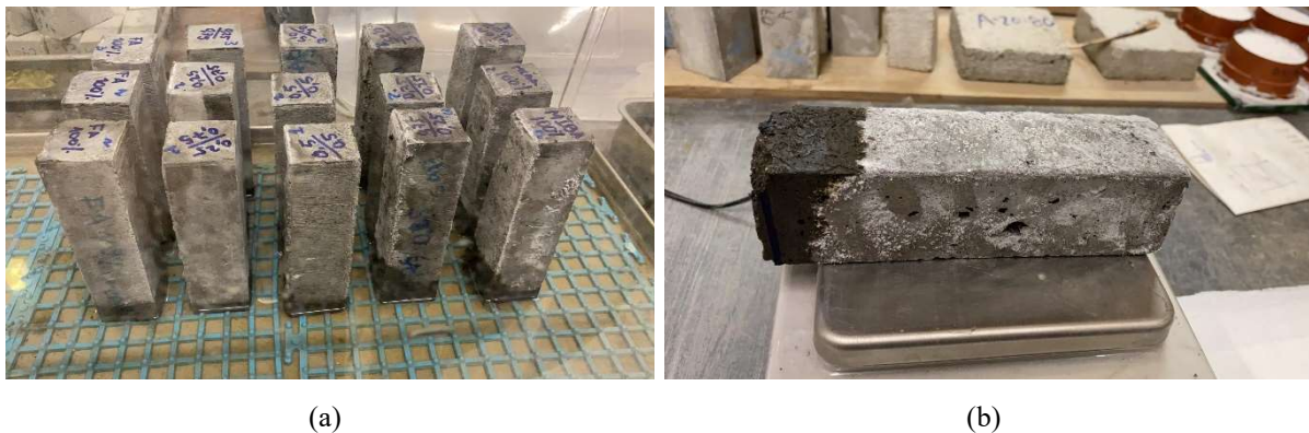
Figure 20 - Capillarity test: (a) experimental setup and (b) 1.0M mortar with loss of mass after 90 minutes
