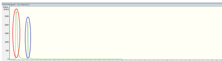
Figure 4.3: Chromatogram of olivetolic acid standard solution analysed with the second HPLC method with injection peak marked with a red circle and with the olivetol peak marked with a blue circle.
