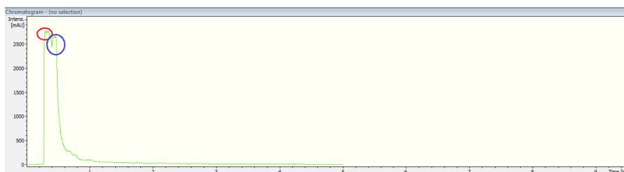
Figure 4.2: Chromatogram of olivetolic acid standard solution analysed with the first HPLC method with injection peak marked with a red circle and with the olivetol peak marked with a blue circle.
