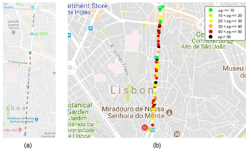
**Figure 4.7:** Representation of all overtaking maneuvers detected in several trips in a specific section of a street (Av. Alm. Reis). (a) Av. Almirante Reis highlighted; (b) Georeference results.
