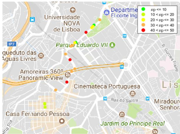
**Figure 3.14:** Georeference of overtaking maneuvers detected for a single trip.
