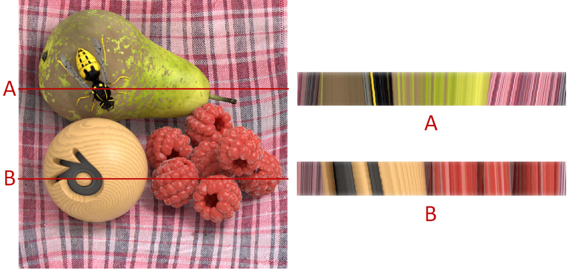
Figure 7.5: Representation of the spatiotemporal characteristics of the EPI. On the left, a static scene from the dataset Still [140] is displayed. This image identifies two horizontal slices that are used to obtain the EPIs. On the right the EPIs obtained from slicing and stacking the sequence of VIs at position A and B are depicted.
