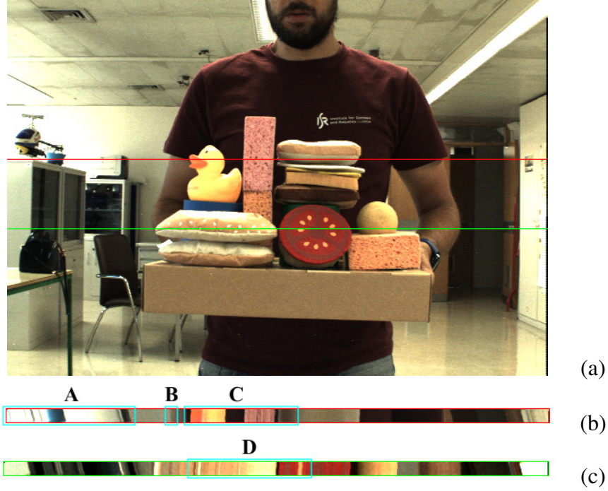
Figure 4.2: The viewpoint cameras identified in red in Figure 4.1.d are used to obtain EPIs from the LF at rows 185 (red) (b) and 265 (green) (c) on the central viewpoint (a).
