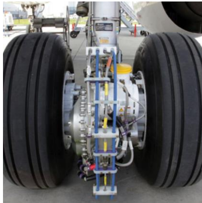
Figure 2. 6- EGTS system. Source: http://www.safranmbd.com/egtstm
