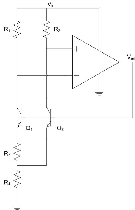
Figure 1.4: Typical bandgap voltage reference.
