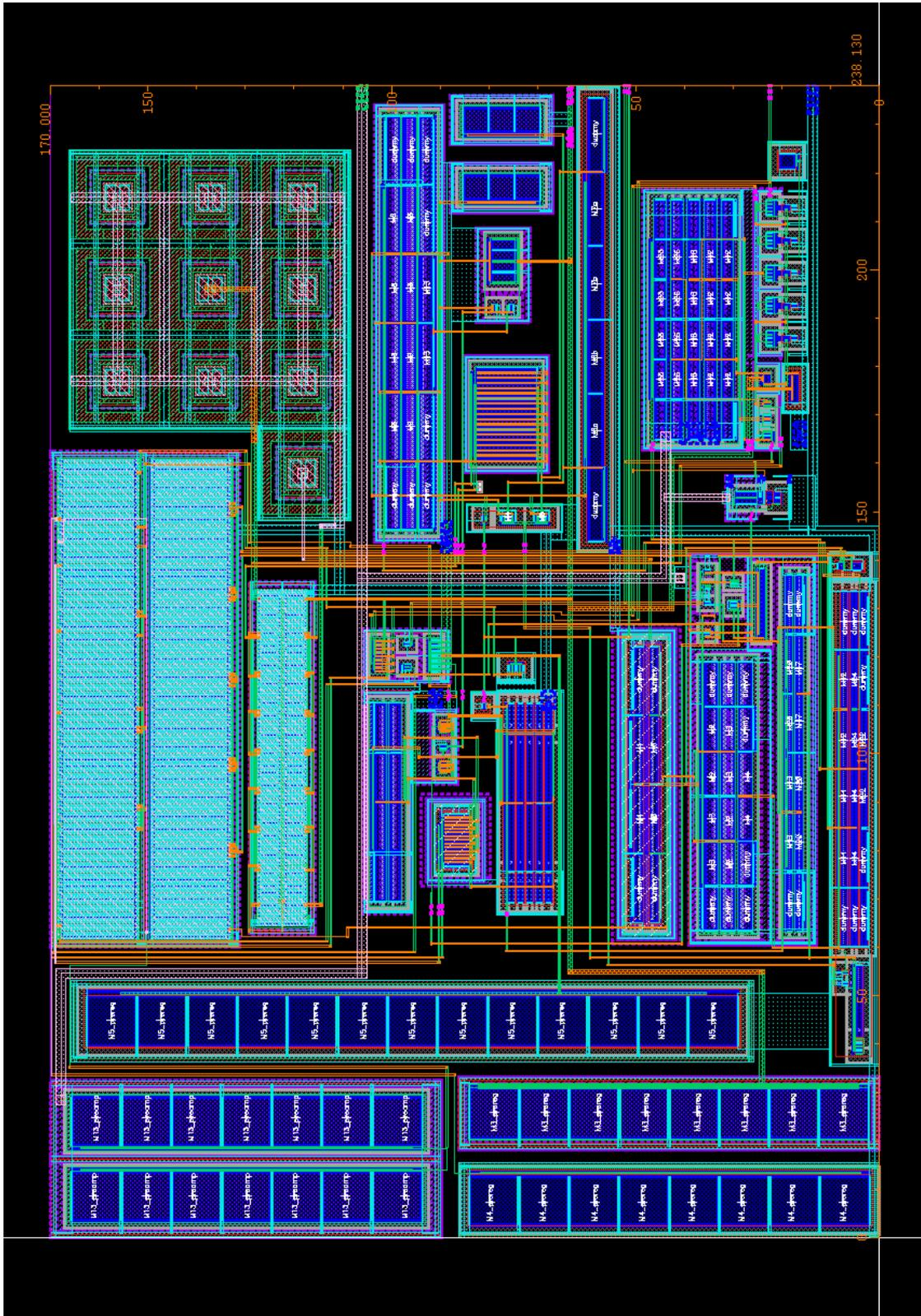
Figure 6.4: Top layout of the proposed bandgap voltage reference.
