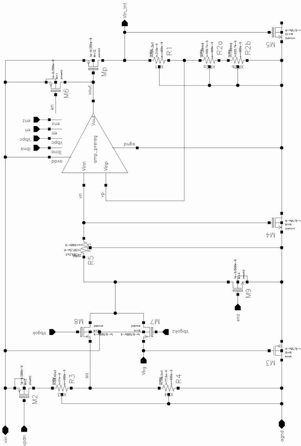
Figure 2.17: Schematic of the pre-regulator: voltage divider, analog multiplexer, error amplifier and pass transistor with the feedback loop.
