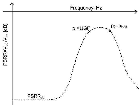
Figure 2.12: PSRR of a conventional linear regulator.
