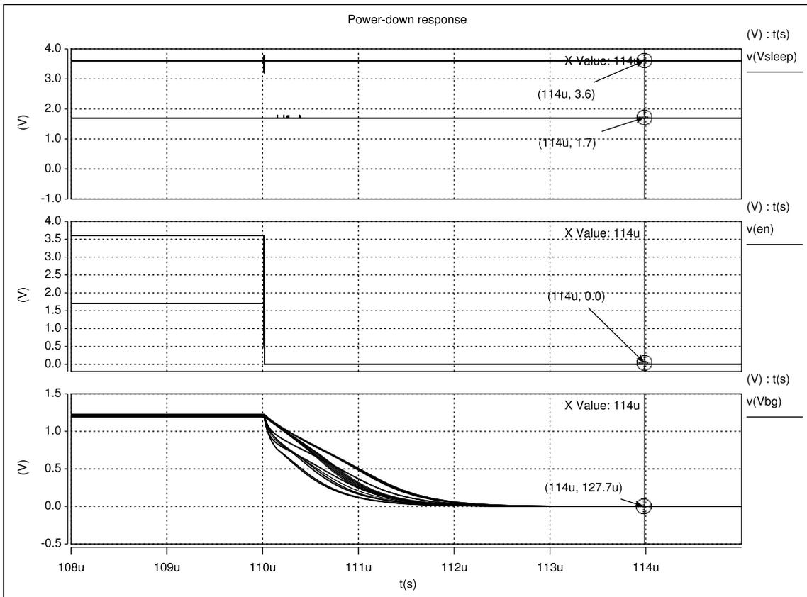
Figure 5.4: Power-down mode of the reference circuit.
