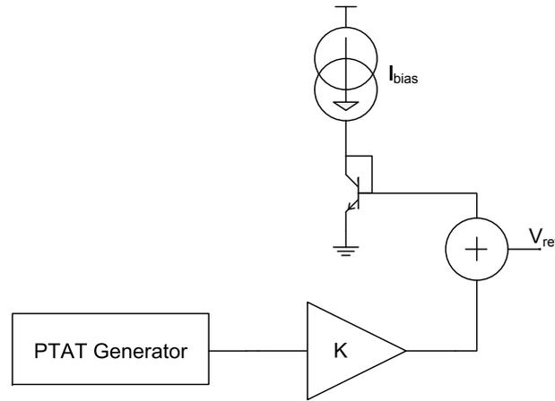
Figure 1.2: Diagram of a bandgap voltage reference.
