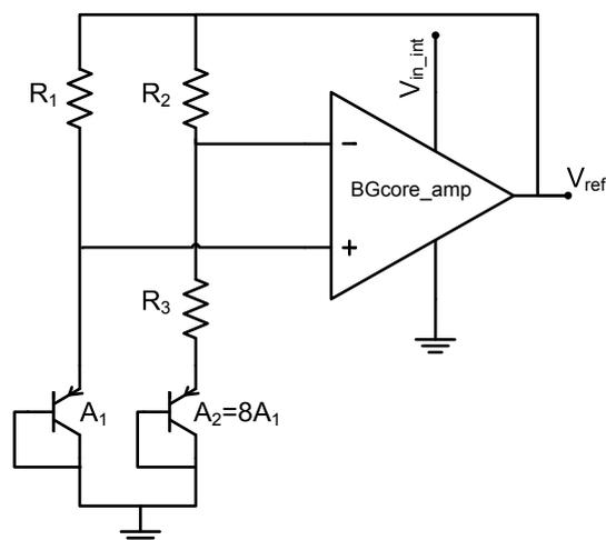
Figure 4.1: Schematic of the proposed architecture for the bandgap reference core.
