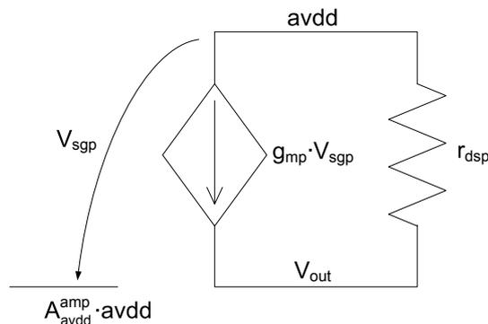
Figure 2.7: Small signal model of the pass transistor considering a PSRR analysis.
