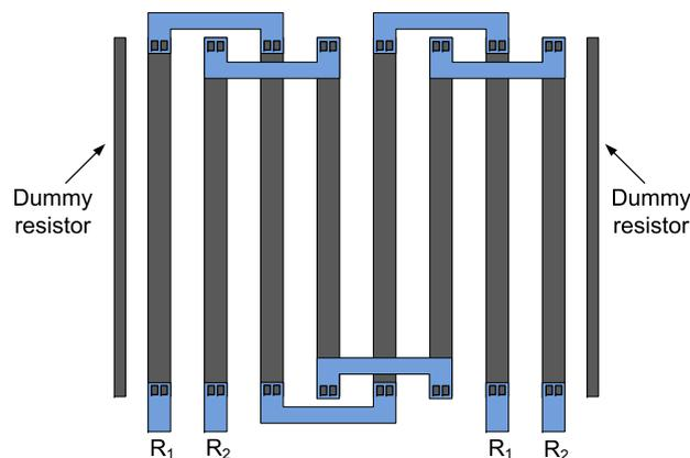
Figure 6.1: Accurate layout for a resistor.
