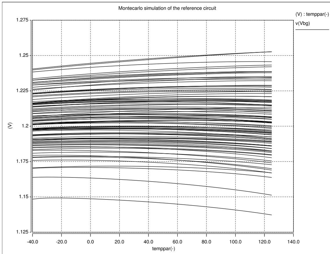
Figure 5.13: Temperature sweep of the reference voltage using Monte Carlo simulation.
