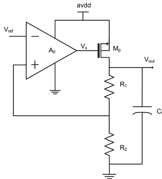
Figure 2.5: A typical topology for a linear regulator.
