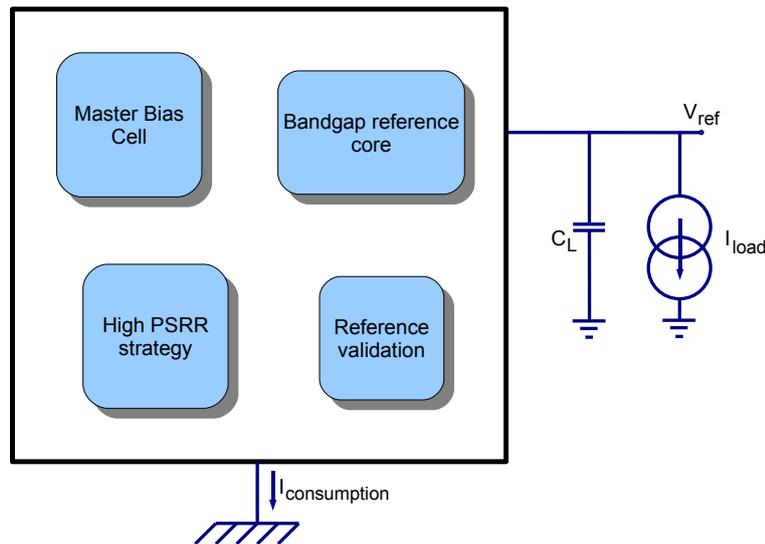
Figure 3.3: Conceptual block diagram of the bandgap voltage reference.
