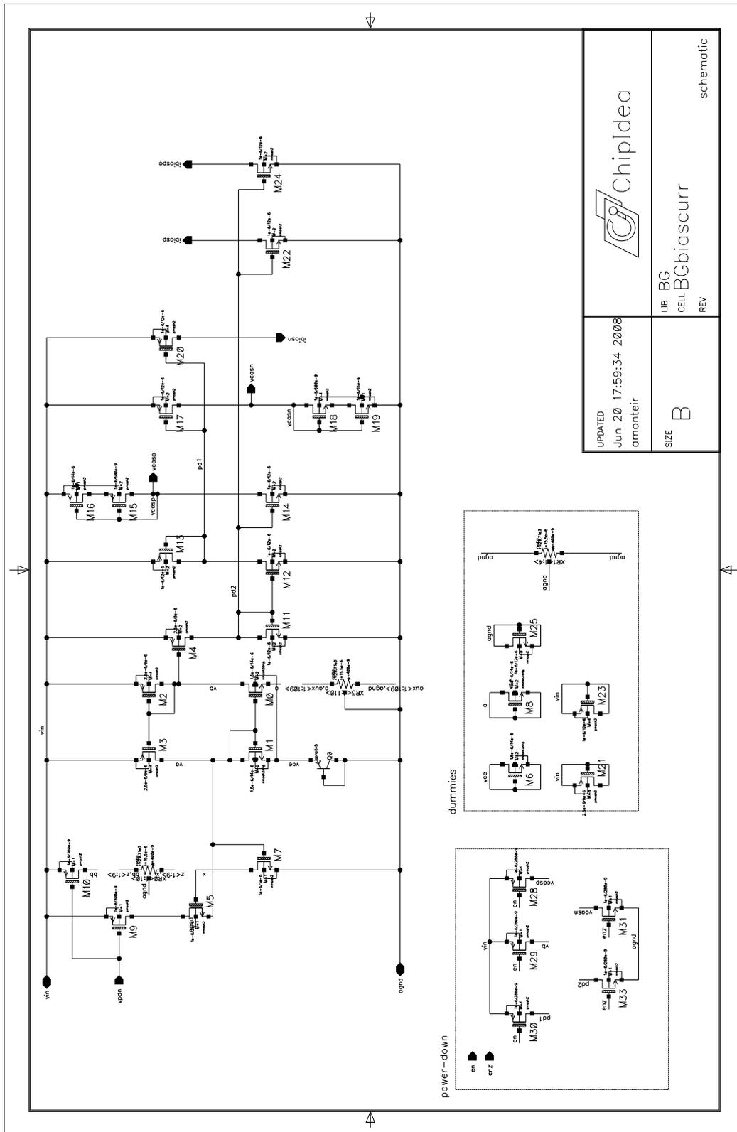
Figure B.4: Schematic of the master bias cell.
