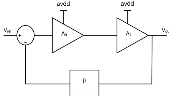
Figure 2.6: Control diagram of the pre-regulator.
