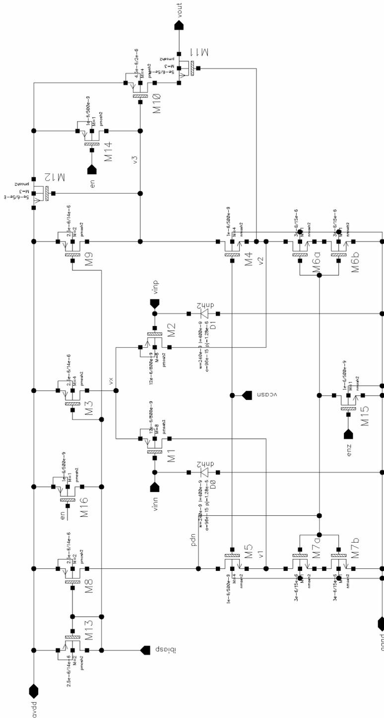
Figure 4.2: Schematic of the error amplifier used in the reference core.
