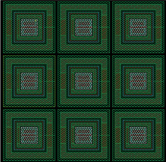
Figure 6.3: Accurate layout structure for the bipolars that reduce mismatching and relative temperature dependence.
