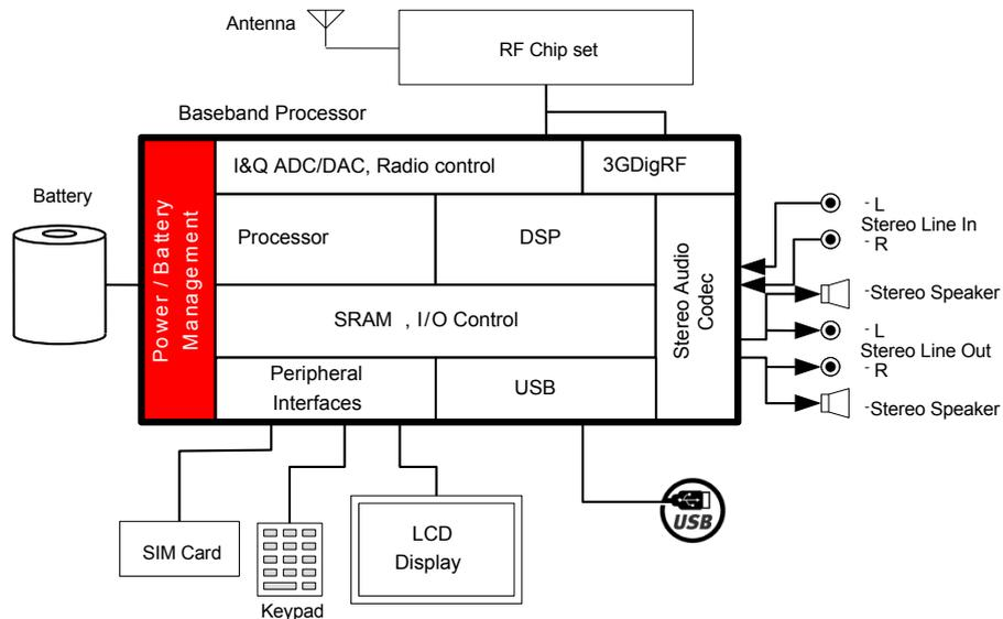
Figure 1.1: Conceptual diagram of the building blocks that constitute a modern System-on-Chip.
