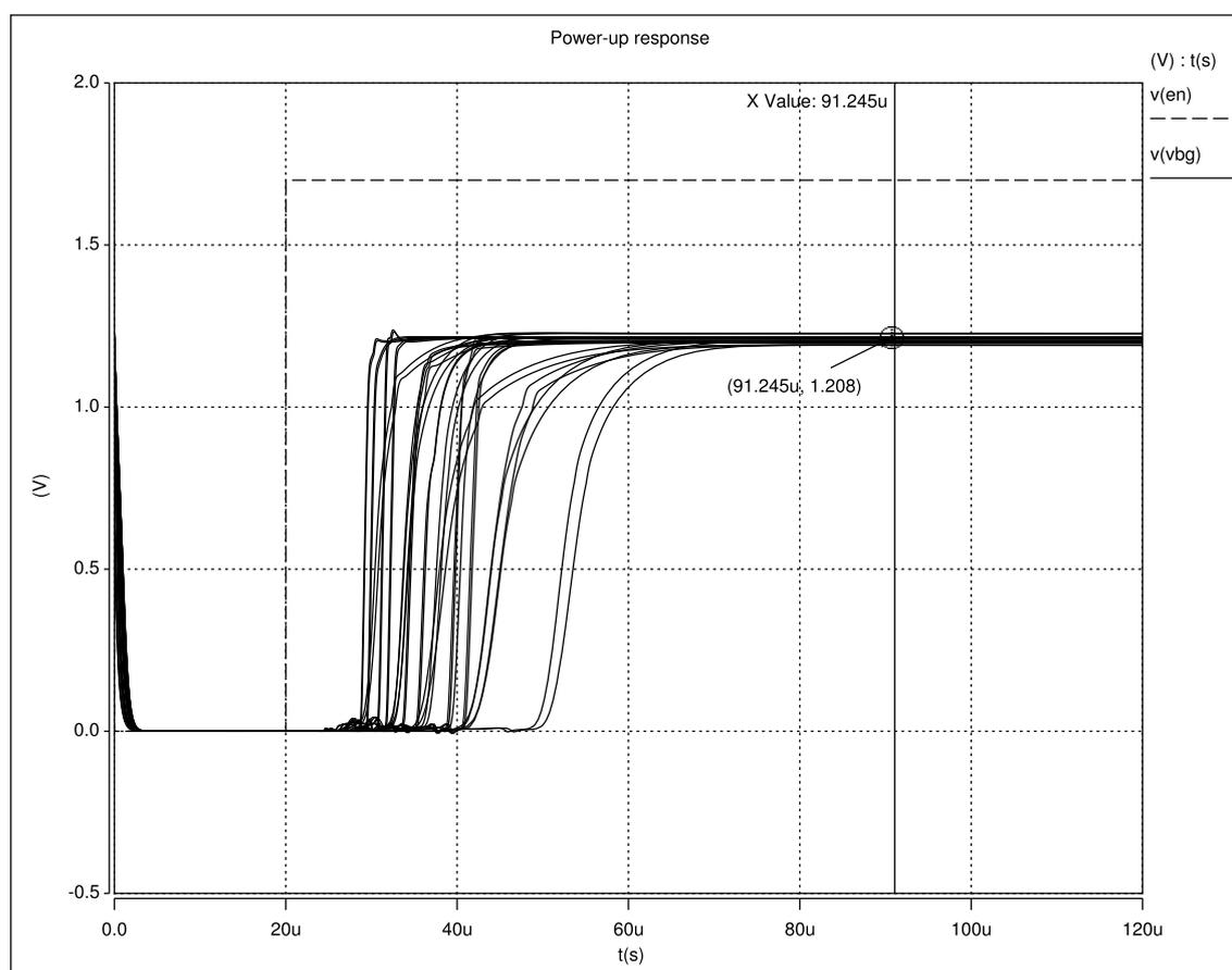
Figure 5.2: Power-up response of the reference circuit.
