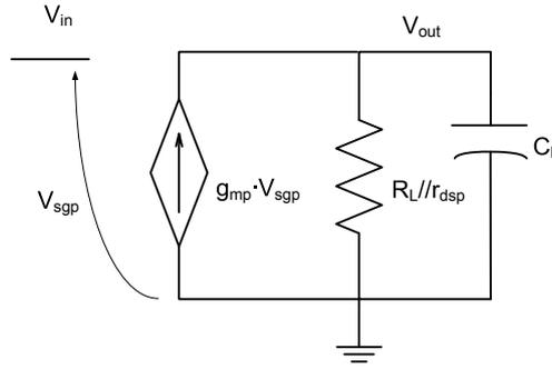
Figure 2.10: Voltage gain of the pass transistor considering a capacitive output impedance.
