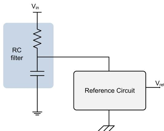
Figure 2.1: State of the Art technique to improve PSRR: use of a RC filter.
