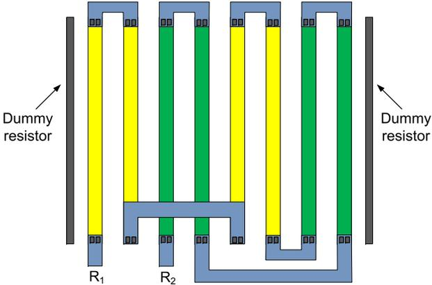
Figure 6.2: Layout for the pre-regulator and master bias cell resistors using only 2 groups of each resistor.
