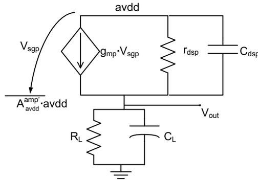
Figure 2.11: Small signal model of the pass transistor considering PSRR analysis.
