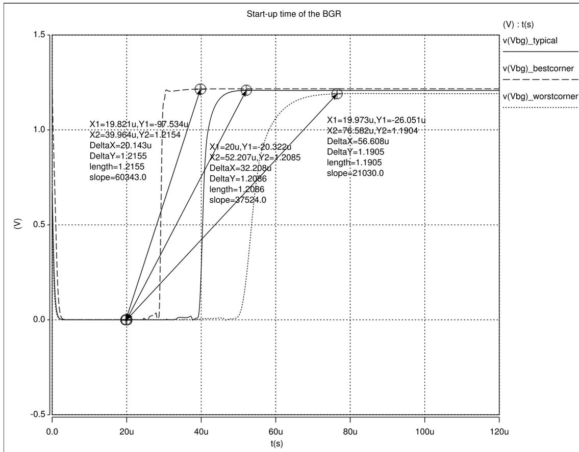
Figure 5.3: Start-up time response of the reference circuit.
