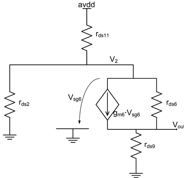
Figure 2.9: Small signal model of the error amplifier in an open-loop configuration.
