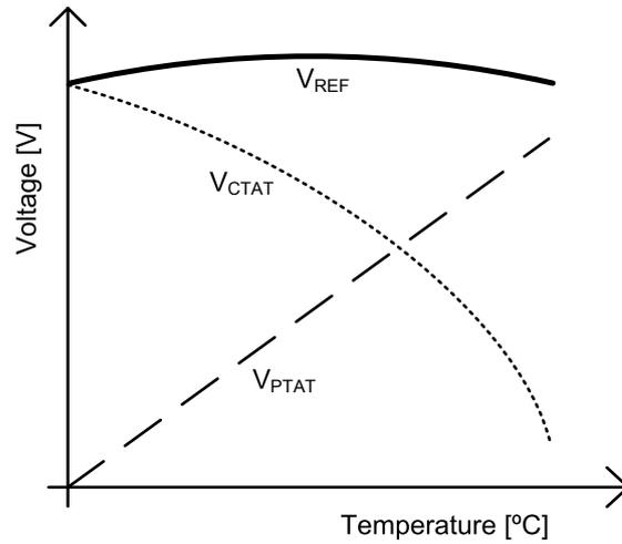
Figure 1.3: Typical temperature curvatures of CTAT, PTAT and bandgap reference voltages.
