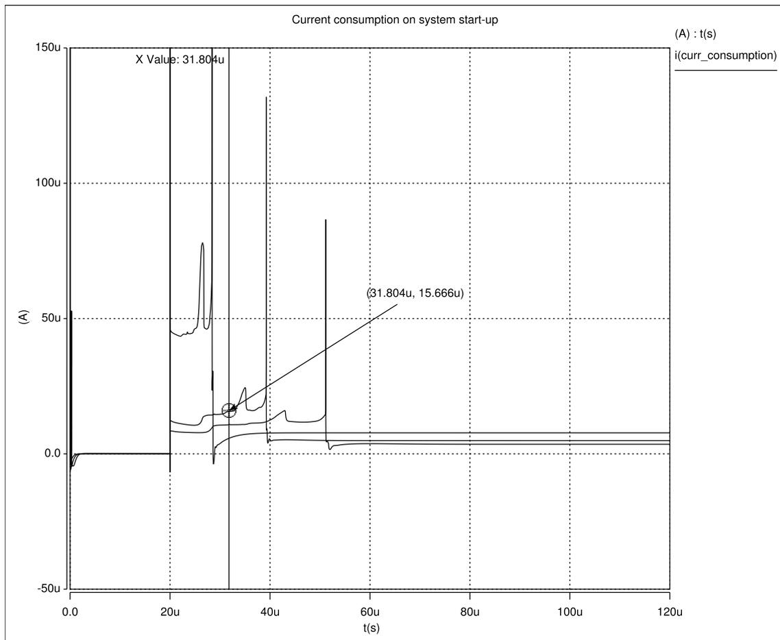
Figure 5.9: Total current consumption during start-up time.
