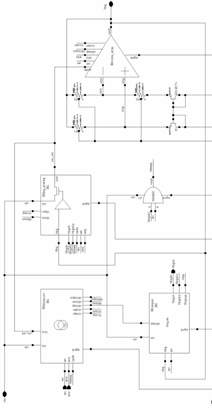
Figure 4.3: Diagram of the proposed bandgap voltage reference circuit.
