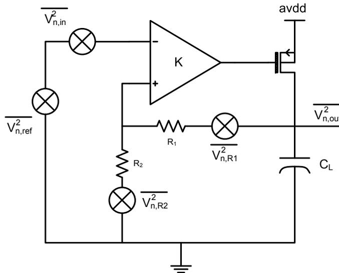
Figure 2.15: Noise sources of a conventional linear regulator.
