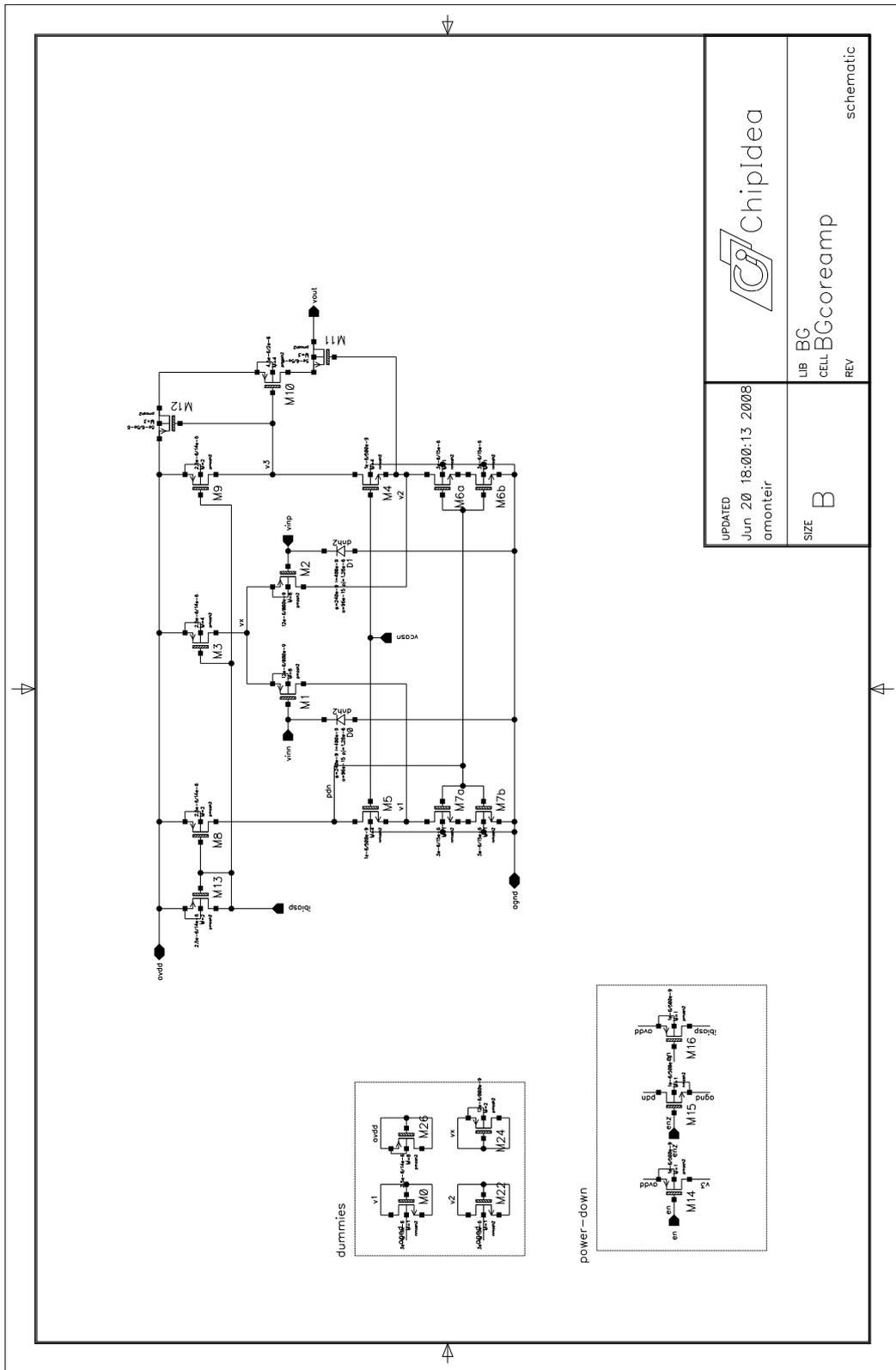
Figure B.5: Schematic of the BGR core's error amplifier.
