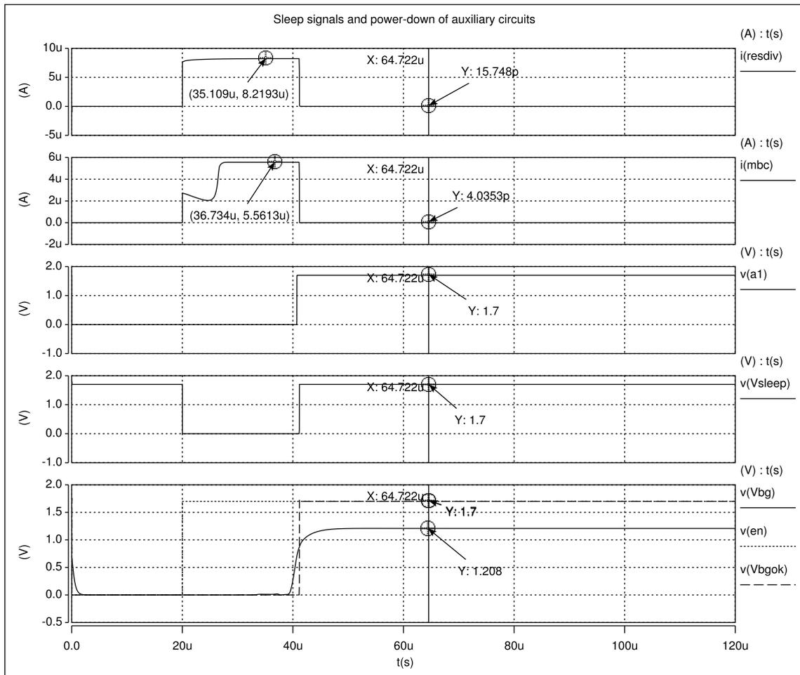
Figure 3.8: Simulation results of the validation signals and sleep mode.
