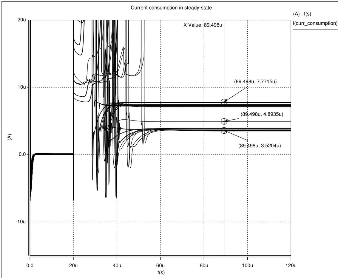
Figure 5.7: Total current consumption in steady-state.
