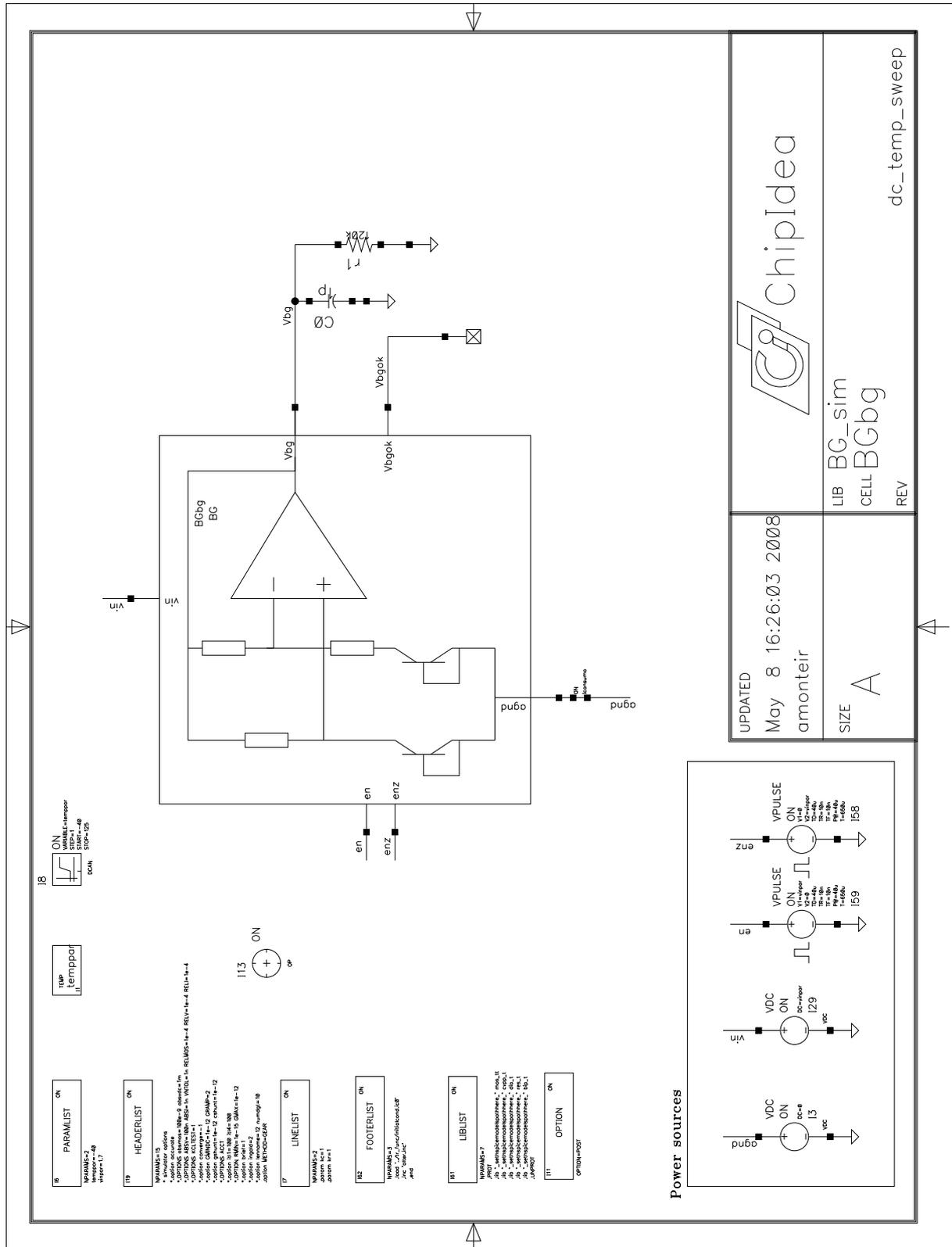
Figure A.3: Testbench used to evaluate the temperature curvature of the BGR.
