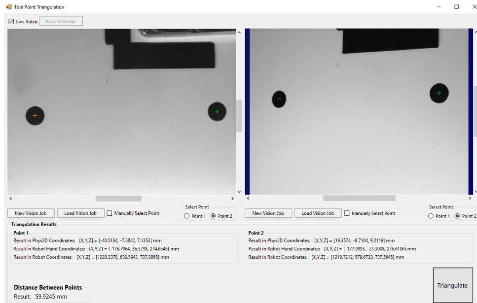
Figure A.8: RoboCalib's tool point triangulation.
