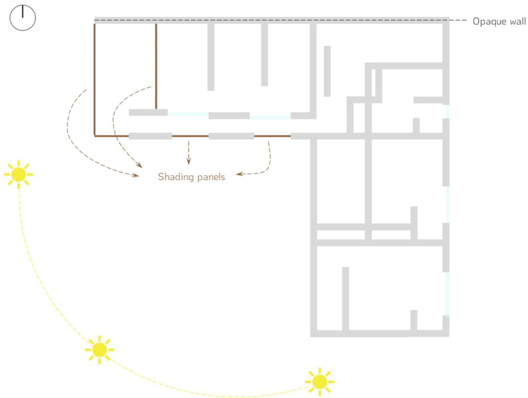
Figure 8.13. Private house conceptual plan and its daylight exposure.
