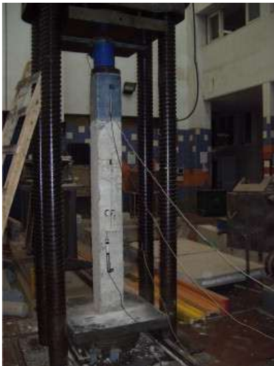
Figure 1.7 - Test set-up of a CFRP reinforced column (Abdel-Hay, 2014).
