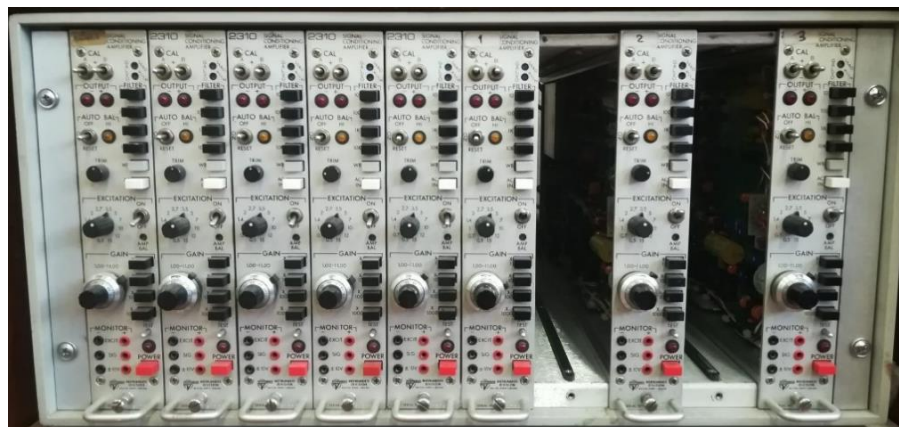
Figure 4-13. Dynamic Wheatstone 2310 Signal Conditioning amplifier.
