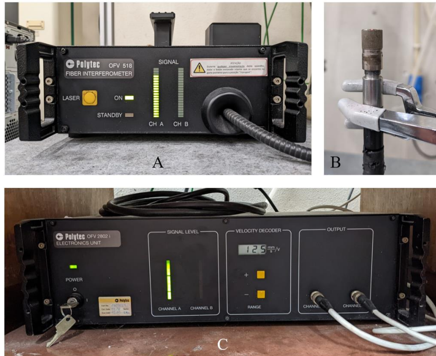
Figure 4-12. Polytec OFV 2802 doppler-vibrometer: (A) fibre interferometer; (B) Laser output lens; (C) Controller electronics unit.
