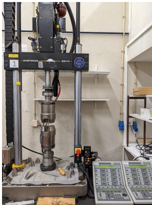
Figure 2-1. Servo-hydraulic tension-torsion fatigue testing machine Instron 8874
