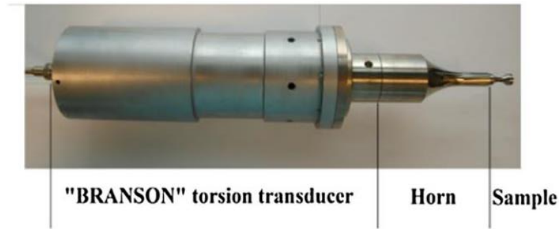
Figure 2-18. A: Nikitin et al. [116] pure torsional machine with a Branson torsion transducer.
