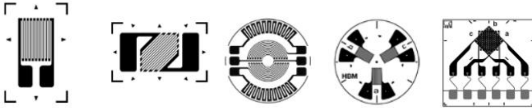
Figure 4-15: Strain gauge examples.
