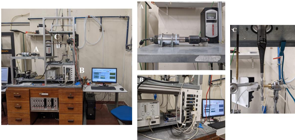
Figure 4-11. Built ultrasonic structure rig and (A) Pure torsion machine; (B) DAQ system; (C) tension-torsion setup with cooling system and temperature pyrometer control sensor.
