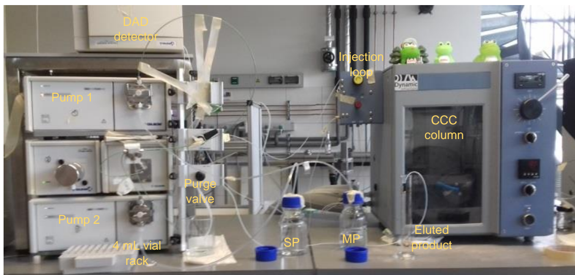
Figure 3.1. CCC apparatus (Dionex Extractions) with a column volume of 18.2 mL, a DAD detector and two HPLC pumps from Gilson (Middleton, USA).
