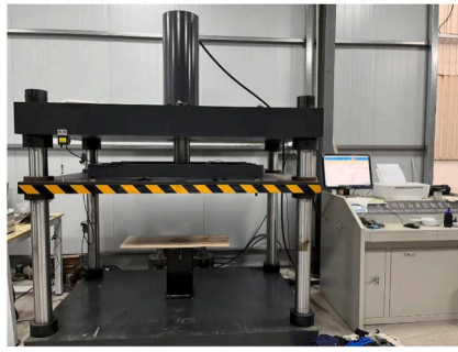
(a) electro-hydraulic servo universal testing
