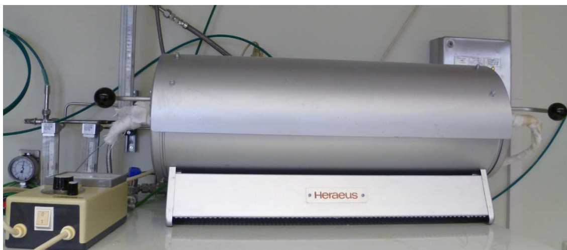
Figure 20 – Cylindrical oven and corresponding temperature controller.
