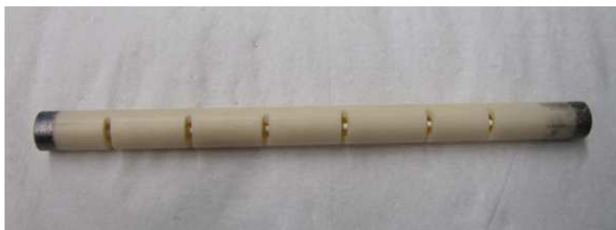
Figure 14 – Nanocomposite-MFI alumina hollow fibre membrane used in this study.
