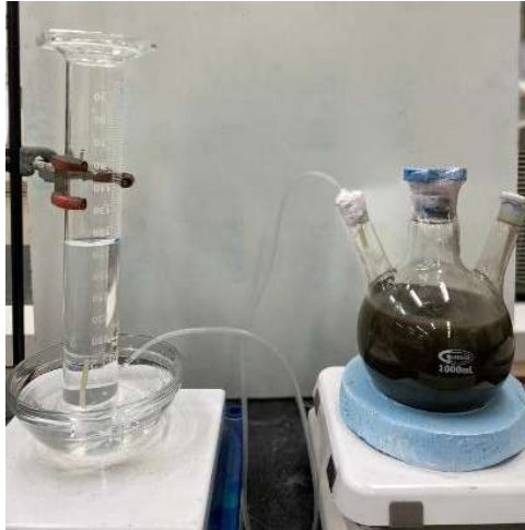
Figure 1. Experimental setup for quantification of metallic aluminium in MIBA.
