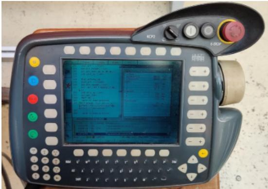
(c) KUKA's remote control console.
