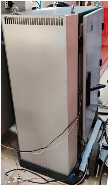
(a) Kuka's main controller unit.
