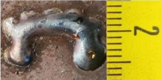
(a) Resulting deposited layer with a lower travel speed in the last deposition section.
