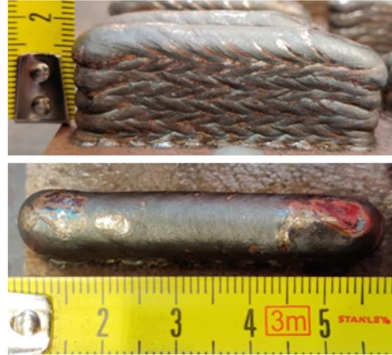
(b) Final straight wall with a horizontal deposition guide line.
