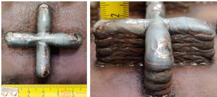
Figure 4.19: Final cross shaped intersection.
