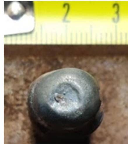
(b) Resulting pin profile using a guide line in the upper part of the pin.
