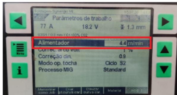
Figure 3.7: Indication of the parameter needed to change the WFS.
