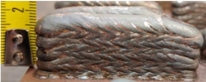
(c) Straight wall aggravated dip, due to the increase of velocity at the end of each layer.
