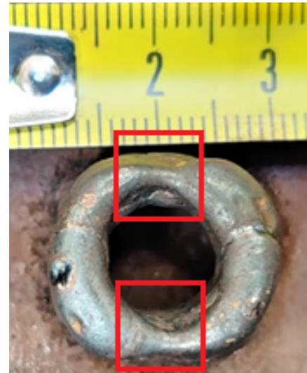
(b) Resulting geometry with less material being deposited in the highlighted areas.
