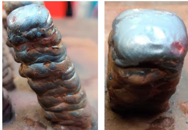
Figure 4.6: Final deposition of a 60° inclined wall, without defects.
