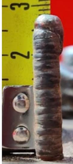
Figure 4.23: Material accumulation at the top of the thin pin, due to the arc ignition delay.
