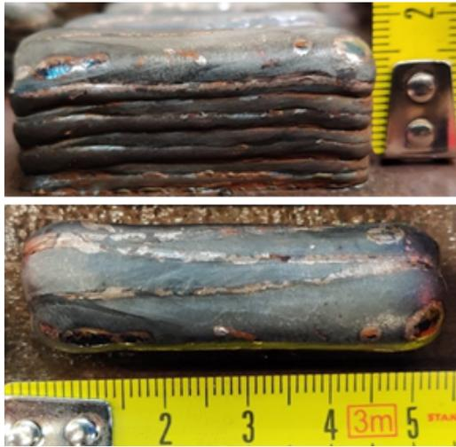
(a) Final straight wall with a vertical deposition guide line.
