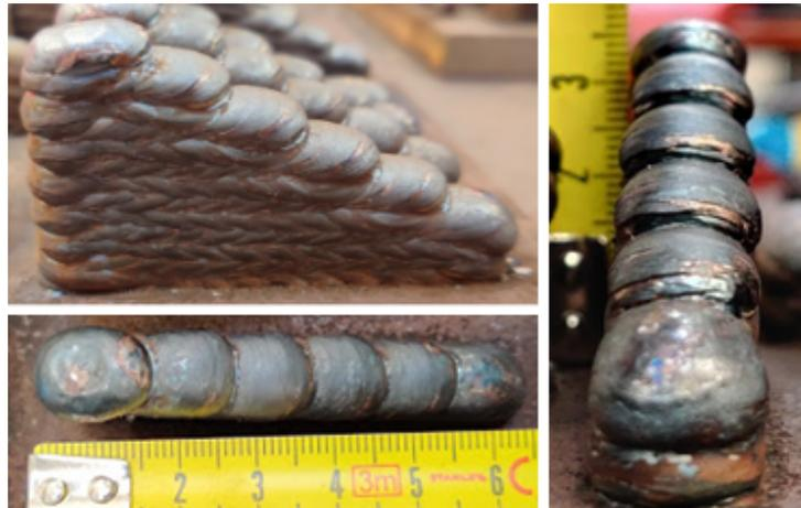
Figure 4.21: Different perspectives on the final staircase vertical increment.
