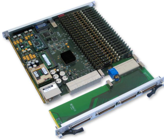
**Figure 5.15:** Photograph of the [IOP](#) board. The board is fully populated with 24 modules, vertically arranged. The rear transmission module with 3 50-pin D-sub connectors for the analog signals and one 37-pin D-sub connector for digital signals is visible on the bottom. Figure available online [[165](#)].
