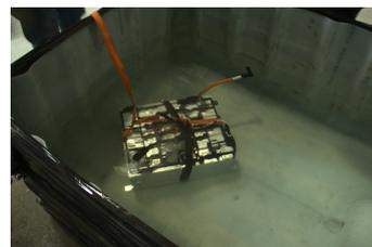
(b) Brine solution used for deactivation at industrial scale.
