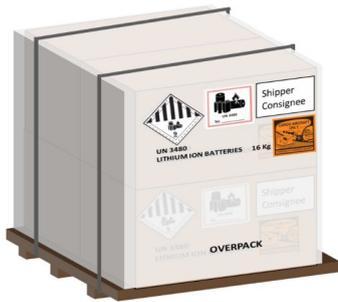
(a) Packaging containing batteries  $\leq 100\text{Wh}$ , overpack Used.
