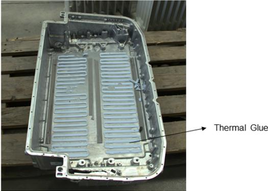
Figure 5.2: Thermal glue on exterior lid of battery pack.
