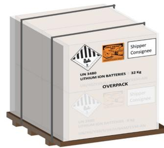
(b) Packaging containing batteries  $>100\text{Wh}$ , overpacked Used.
