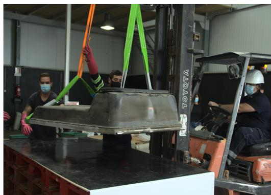
Figure 5.1: Placing battery pack onto workstation using forklift.
