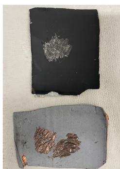
(a) Scrubbed electrode foils: anode [bottom], cathode [top].
