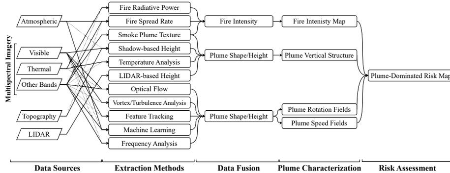
**Fig. 2.** High-level architecture of the proposed methodology. In the *Data Sources*’ section, solid lines indicate primary sources, while dashed lines represent secondary (optional) sources. *Other Bands* include Near Infra-Red, Infra-Red and Red Edge.
