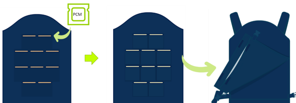
Figure 5. Study of the integration of PCM packages in the vest
