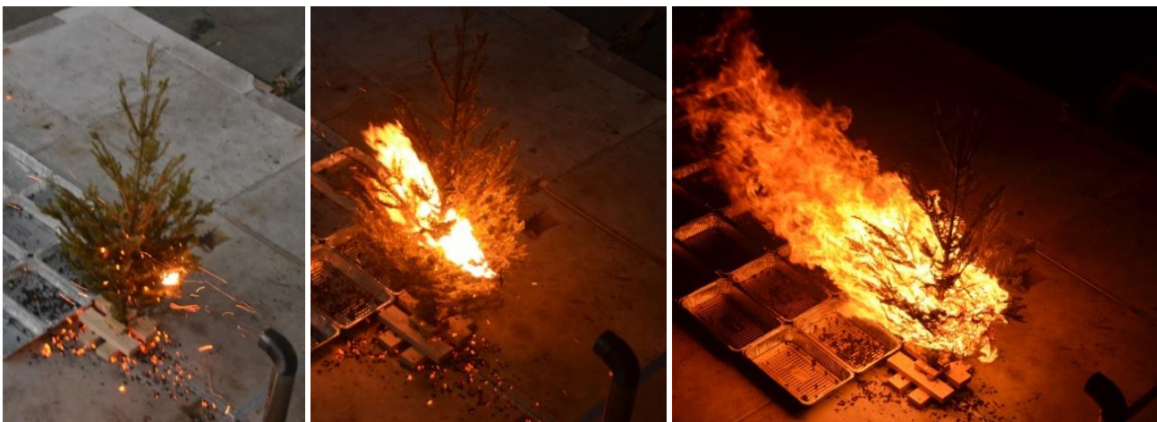
Figure 2- Douglas-fir tree ignited by the firebrand generator under a 4 m/s wind
