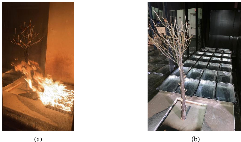
Fig. 2: Testbed. (a) Propane burner. (b) Mounting platform and aluminum pan array used to collect the firebrands generated
