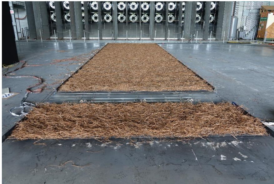
Figure 1 – Fuel bed with pine straw fuels and discontinuous fuel gap layout at IHBS wind tunnel
