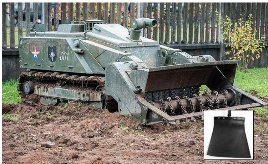
Fig. 5 Uran-6 unmanned multifunctional demining system (Army 2021)
