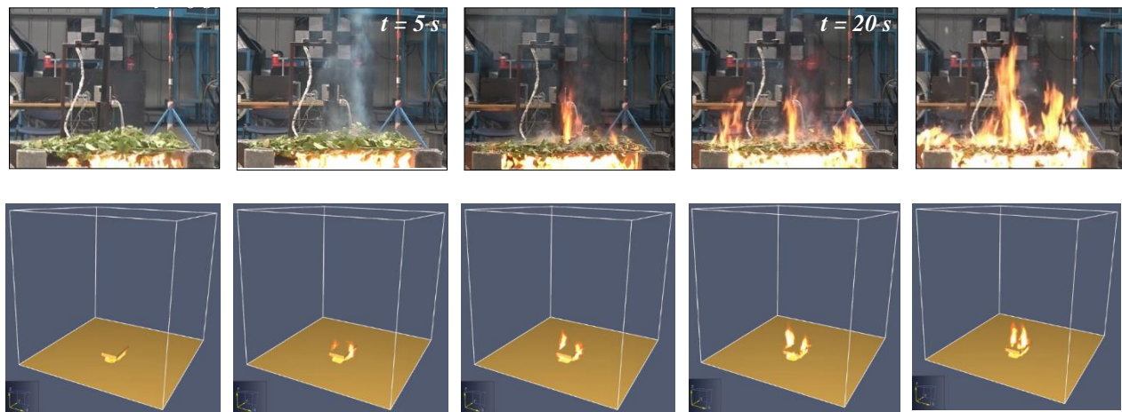
Figure 8. Comparison of the real-time lab experiments with numerical modeling from FDS for the Grapevine plant at 0; 5; 15; 20; and 40 s.
