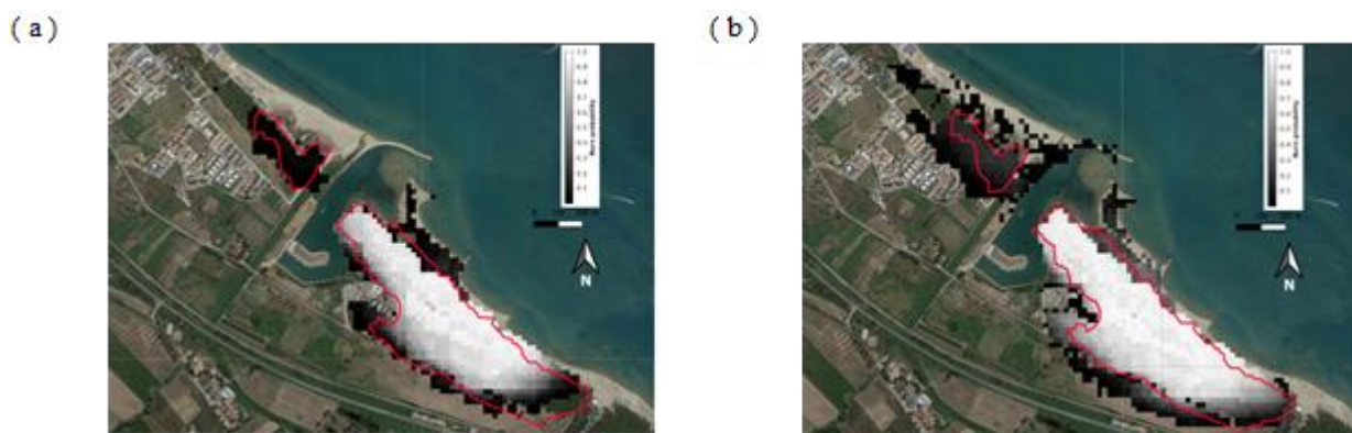
Figure 4- Computed burn probability map with the Perryman parametrization implemented. Figure 4-(a) shows the burn probability after 3 hours and Figure 4-(b) after 5 hours.
