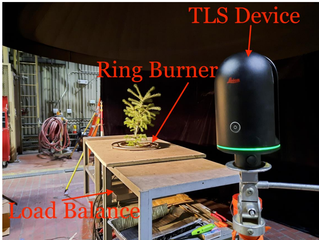
Figure 1- Experimental setup with LIDAR scanner at the Missoula Fire Sciences Laboratory
