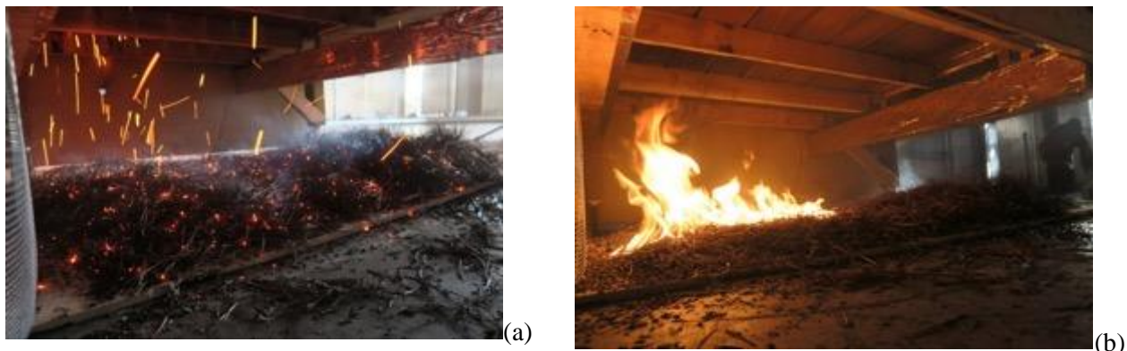
Figure 3. Ember penetration through gaps between deck boards; (a) embers falling to ground and (b) resulting in the ignition of pine needles that accumulated under the deck.
