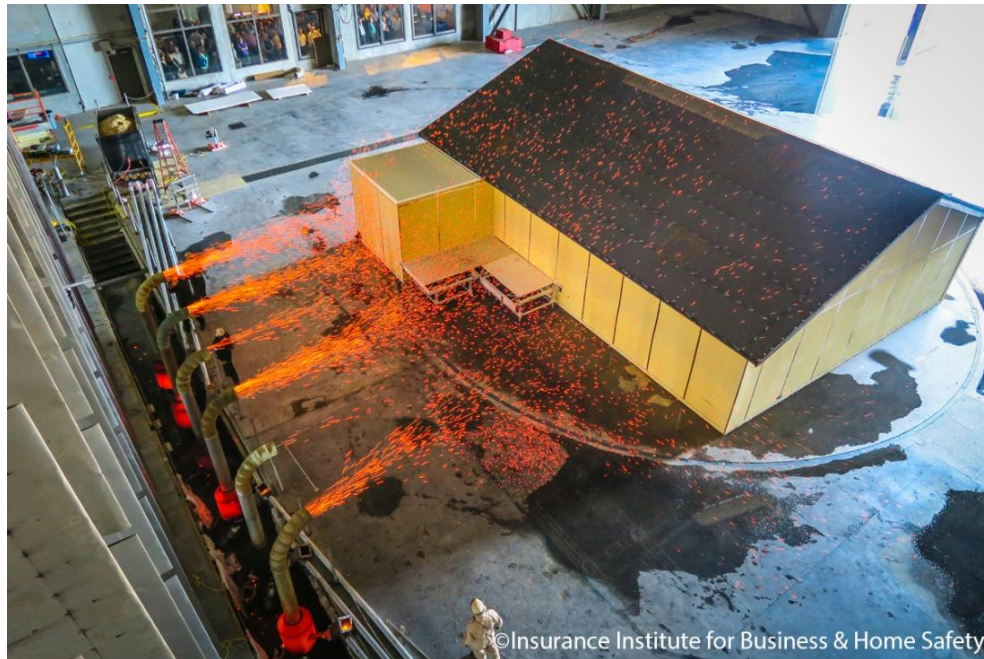
Figure 4. Test building and ember generator system used in the accumulation study. As shown, the collection trays were initially covered with a solid panel until steady flow from the generators was observed.
