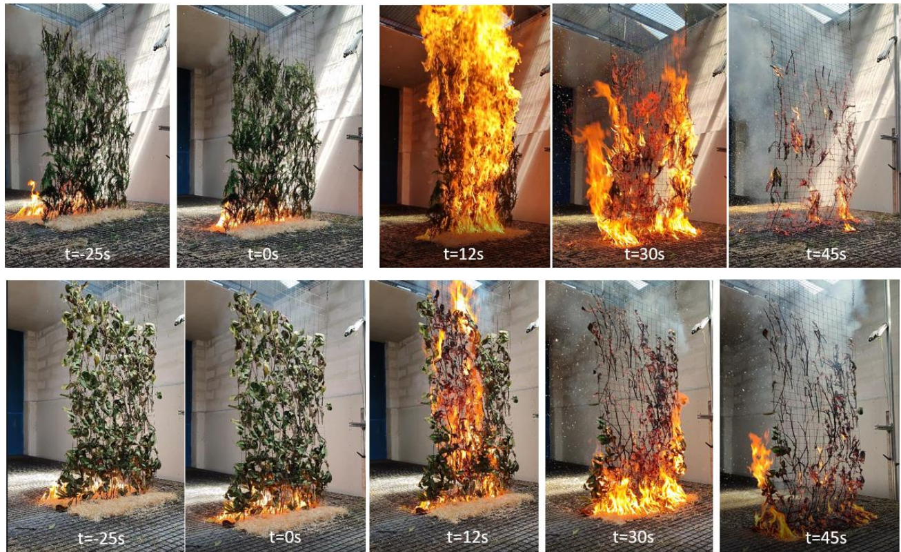
Figure 6 – Fire contaminating from excelsior fire to the hedge under zero-wind conditions, (upper) for cypress and (lower) for oleander. Propagation visualized in 5 phases (from left to right): excelsior fire approaches, excelsior fire at the foot of the hege (reference time t=0s ), fire at maximum development in the hedge, fire largely decreasing, fire in extinction phase
