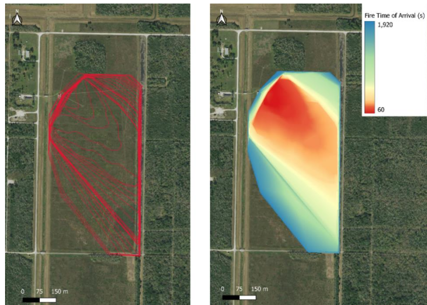
Figure 3. Fire progression during the FireFlux II experiment (Clements et al., 2019) derived from airborne IR imagery. Left: fire perimeter at 60-s intervals. Right: fire time of arrival at every location in the burn unit, relative to the time of ignition. Base image provided by the USDA National Agriculture Imagery Program.
