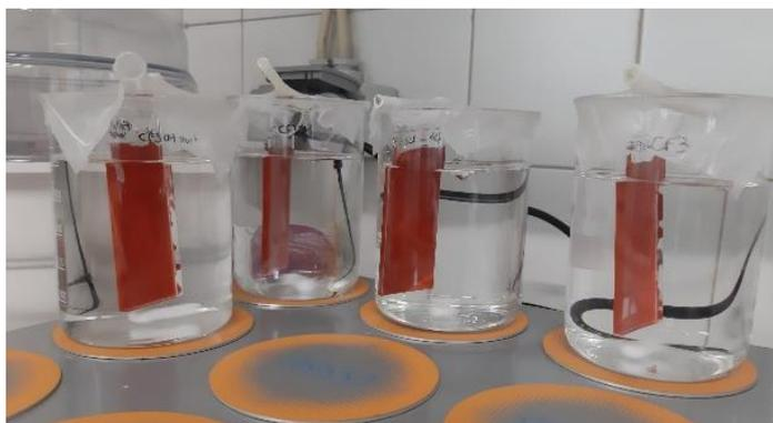
**Figure 5.** Leaching test of panels coated with the optimised formulations containing the compounds **7**, **9** and **11** and control coated reference panel submerged in distilled water.
