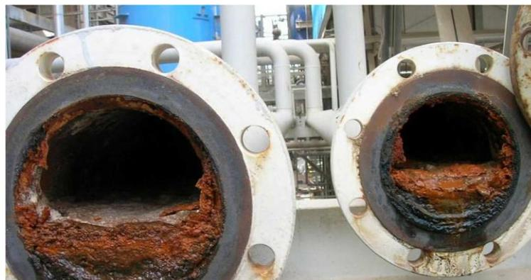
**Figure 3.** Biofouling on a cooling water pipe in the ship's system.<sup>[25]</sup>
