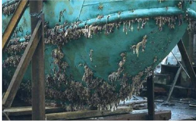
**Figure 2.** Biofouling on a ship's hull. Courtesy of Hempel's Marine Paints A/S.<sup>[24]</sup>
