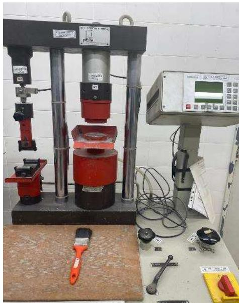
Figure 15 - Equipment to determine flexural strength and compression strength of mortars
