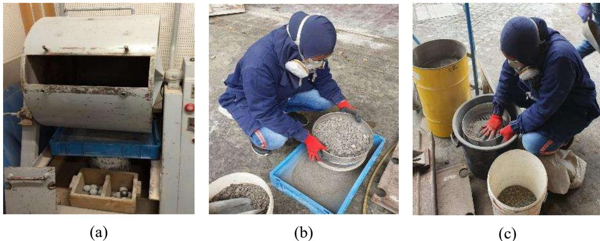
Figure 4 - (a) Grinding in the Los Angeles machine; (b, c) size separation through sieve N. 4
