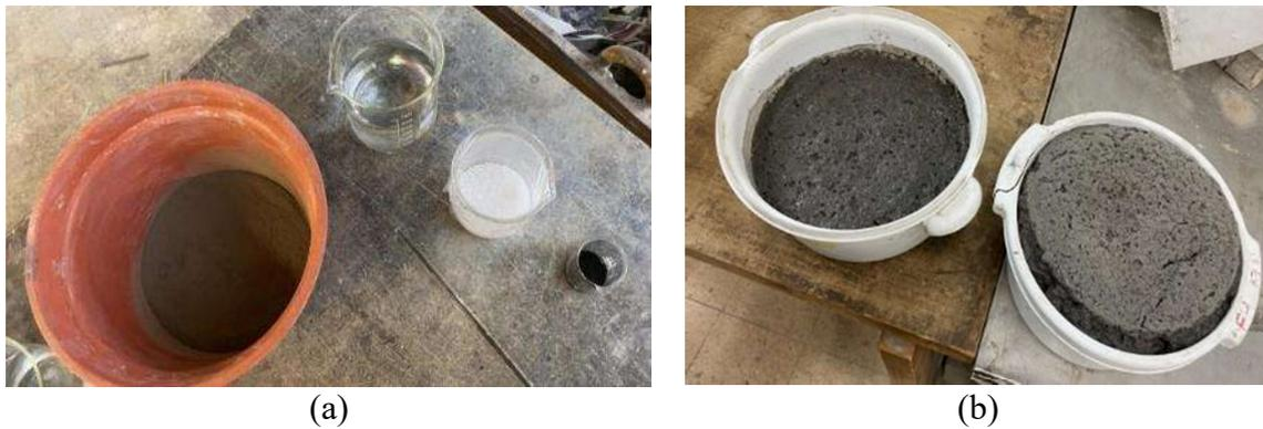
Figure 7 - (a) Materials for the preparation of AAM; (b) reaction of MIBA and NaOH
