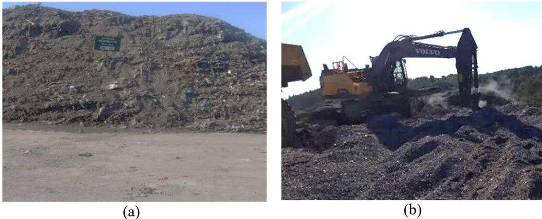
Figure 1 - (a) MIBA stacks separated by generation month; (b) MIBA sampling
