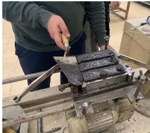
Figure 3: Excess layers of mortar removed from the top surface
