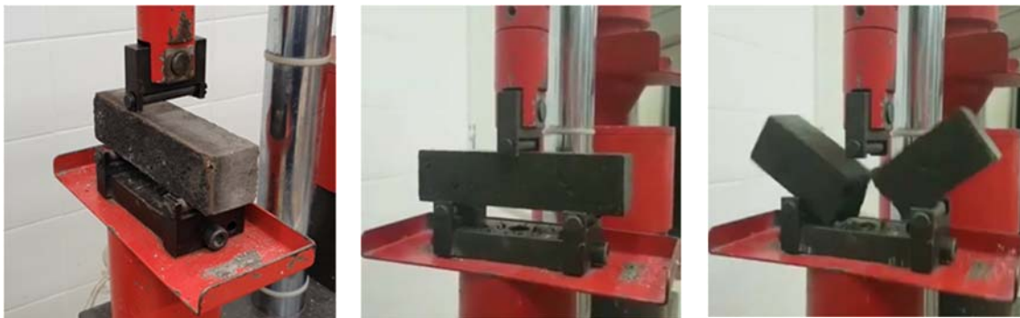
Figure 5. Table 10 shows the equipment used for flexural strength, procedure, and equations according to EN 1015-11 [6].
