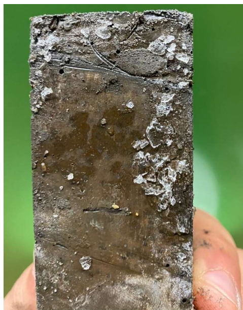
Figure 5 - Efflorescence caused by \text{Na}_2\text{CO}_3
