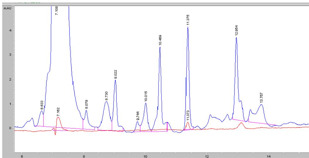
**Figure 37:** Chromatogram of hydrogenations in autoclave at 224°C, 34bar and 2 hours of hydrogenation.
