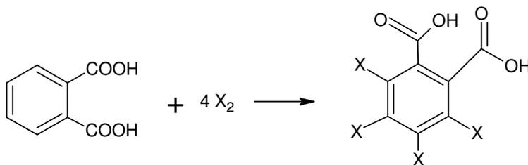
**Figure 5:** Halogenation of phthalic acid.
