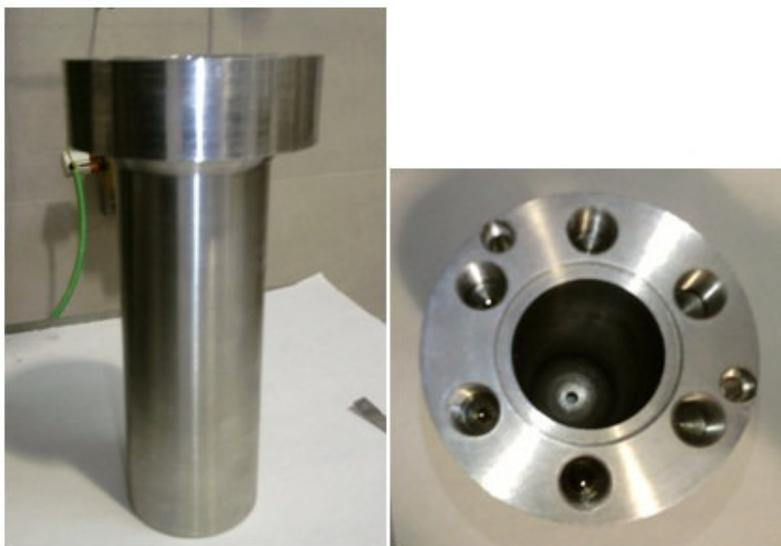
**Figure 16:** Autoclave reactor of hydrogenation.
