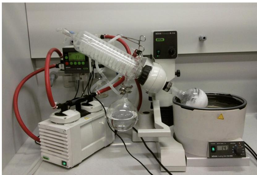
**Figure 22:** Rotary-evaporator used to recover PIPA from dimethylformamide.
