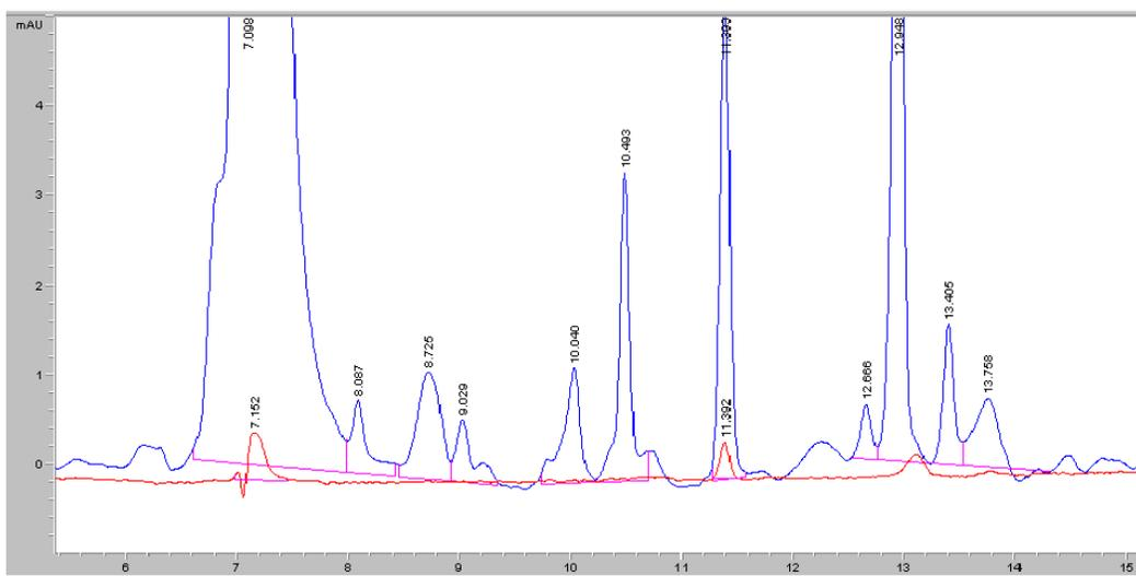
**Figure 39:** Chromatogram of hydrogenations in autoclave at 237°C, 30bar and 2 hours of hydrogenation.
