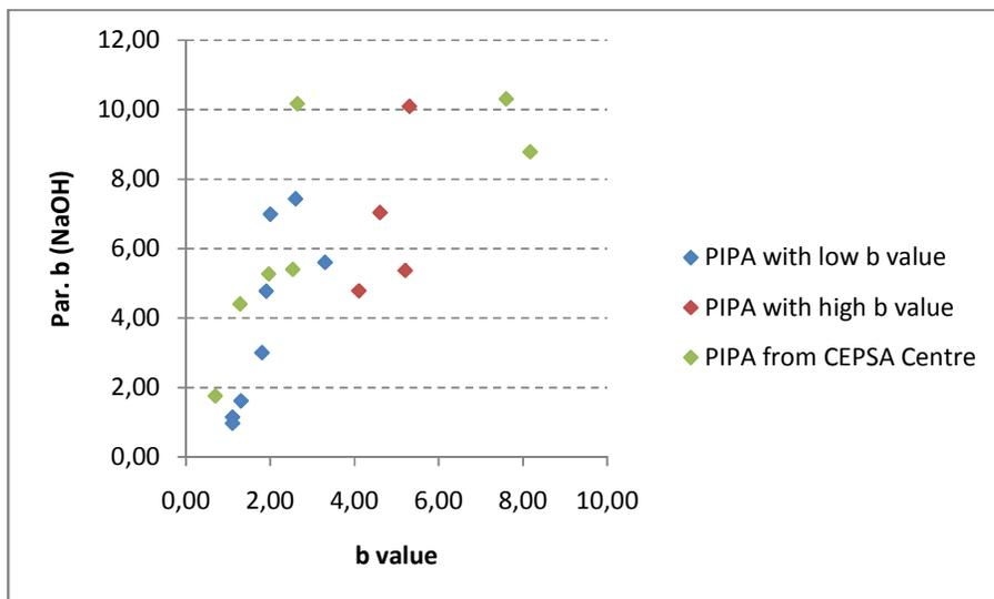
Figure 29: Relation between Parameter b (with NaOH) and *b* value.
