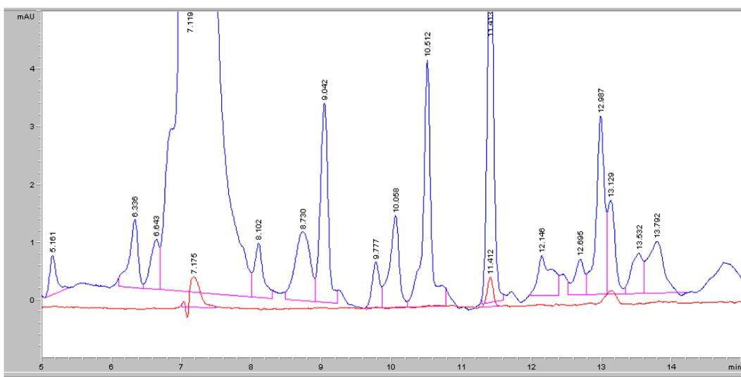
**Figure 42:** Chromatogram of hydrogenations in autoclave at 224°C, 34bar and 1 hours of hydrogenation.
