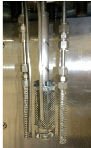
**Figure 20:** Inside of the reactor - Catalyst's basket, thermocouple and basket with glass spheres.
