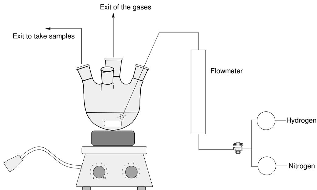
**Figure 13:** Scheme of hydrogenations at semi-continuous.
