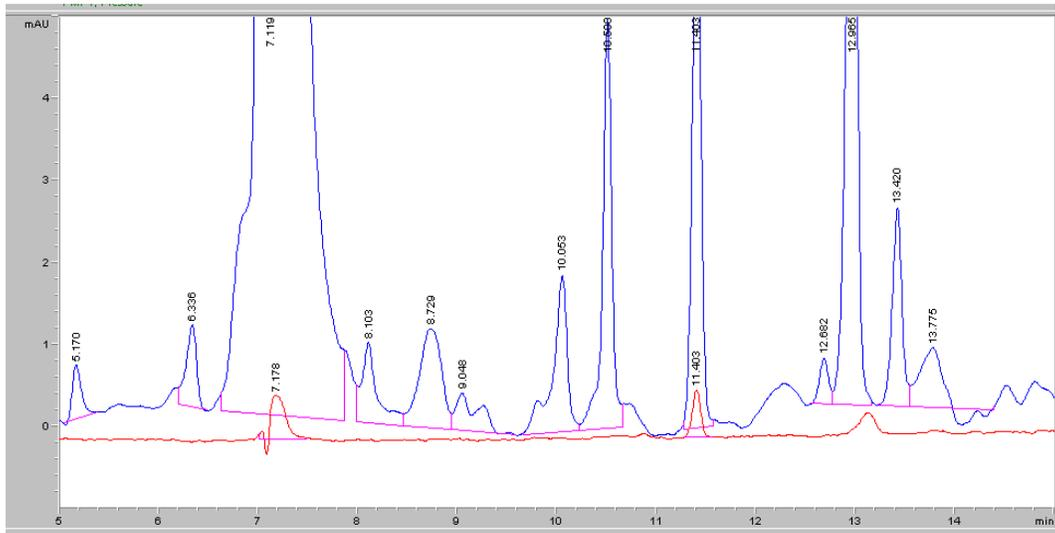
**Figure 43:** Chromatogram of hydrogenations in autoclave at 237°C, 38bar and 1 hours of hydrogenation.
