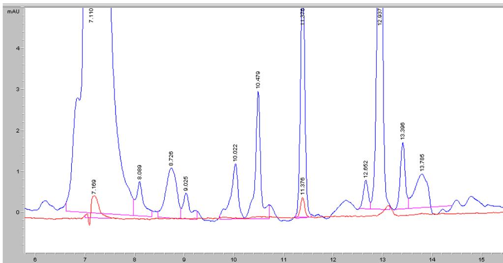
**Figure 41:** Chromatogram of hydrogenations in autoclave at 212°C, 30bar and 2 hours of hydrogenation.
