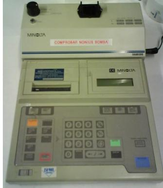
**Figure 24:** Minolta Chroma Meter CT-310, used to measure the *parameter b*.
