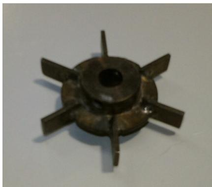
**Figure 21:** Impeller from the hydrogenation reactor.
