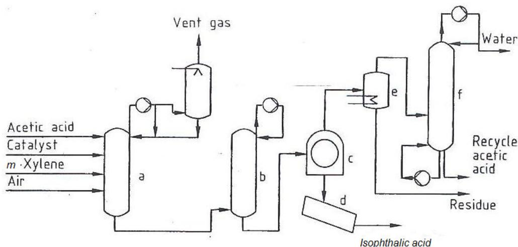
**Figure 8:** Catalytic, liquid-phase oxidation of *m*-xylene to isophthalic acid by the Amoco process. a) oxidation reactor; b) surge vessel; c) filter; d) dryer; e) residue still; f) dehydration column [3].
