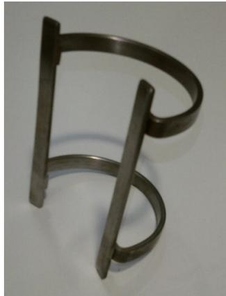
**Figure 19:** Baffle of the reactor.
