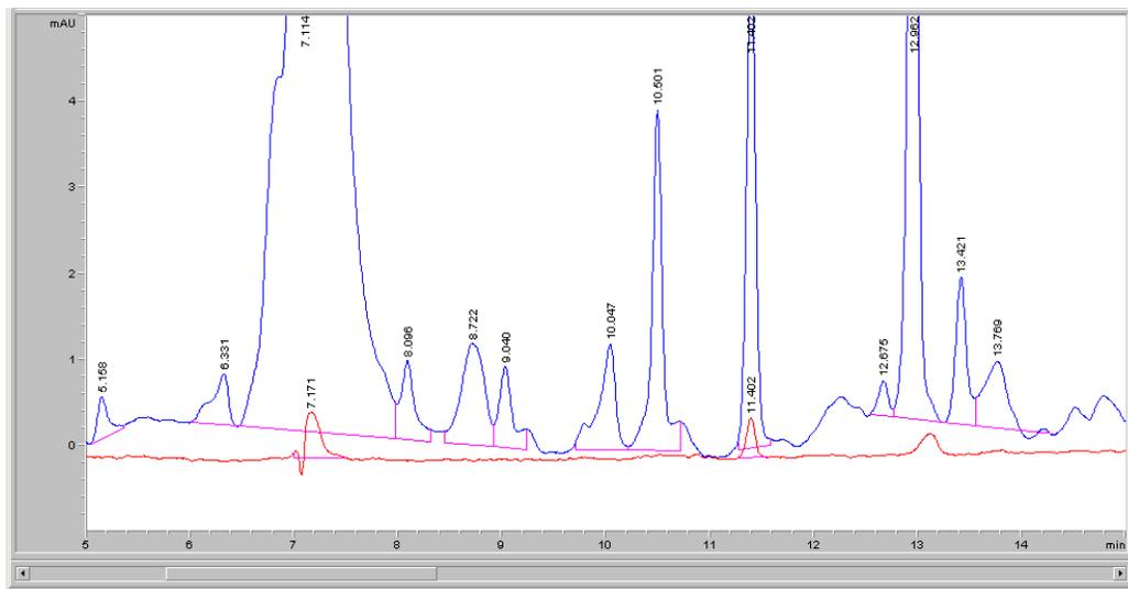
**Figure 44:** Chromatogram of hydrogenations in autoclave at 237°C, 30bar and 1 hours of hydrogenation.
