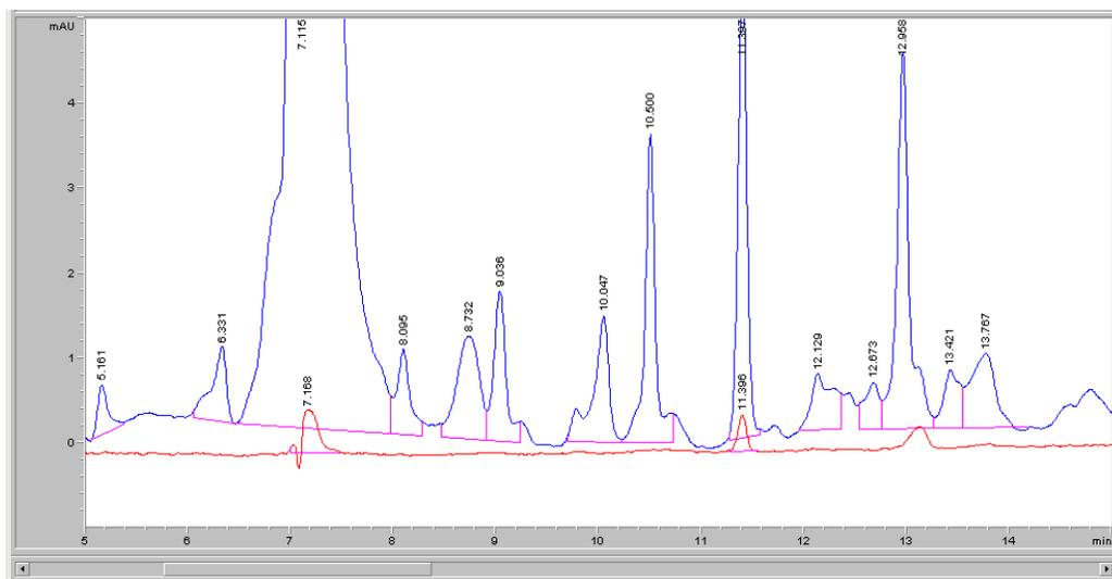
**Figure 45:** Chromatogram of hydrogenations in autoclave at 212°C, 38bar and 1 hours of hydrogenation.
