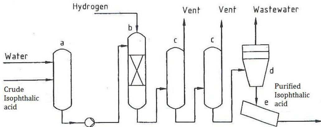
**Figure 11:** Purification of Isophthalic acid by the Amoco process. a) Slurry drum; b) Hydrogenation reactor; c) Crystallizers; d) Centrifuge; e) Dryer [3].
