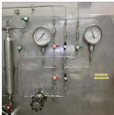
**Figure 15:** System of gases in autoclave's system.
