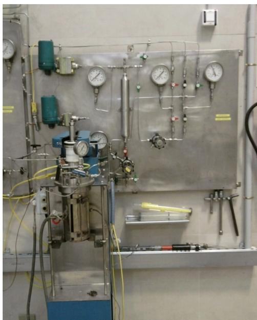
**Figure 14:** System of autoclave.
