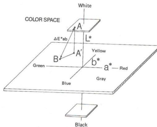
**Figure 25:** Scheme of measure units of colorimetry (A – target colour; B – specimen’s colour; A’ – target colour at the same lightness level as specimen’s colour).
