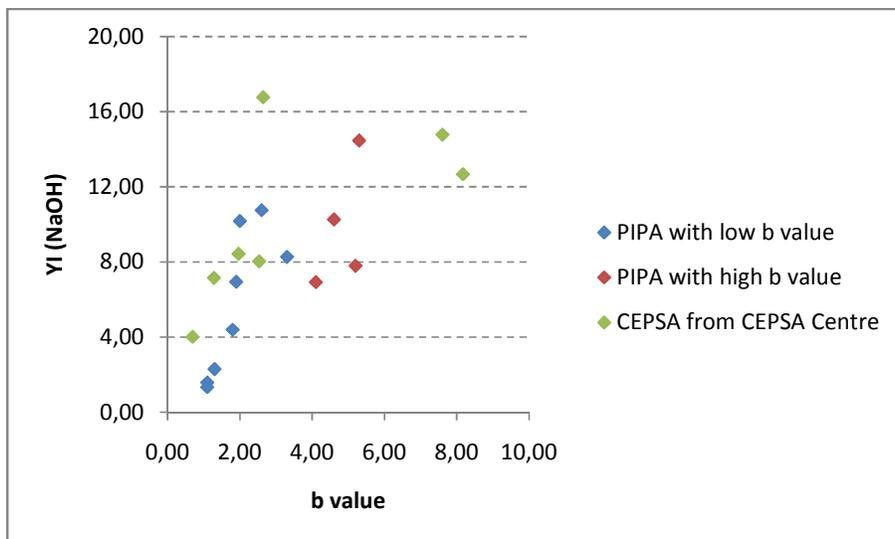
**Figure 31:** Relation between yellow index (with NaOH) and the *b* value.
