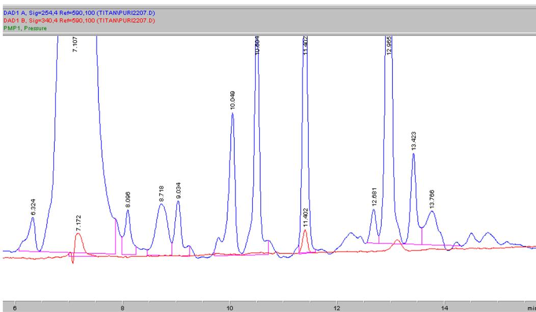
**Figure 40:** Chromatogram of hydrogenations in autoclave at 212°C, 38bar and 2 hours of hydrogenation.
