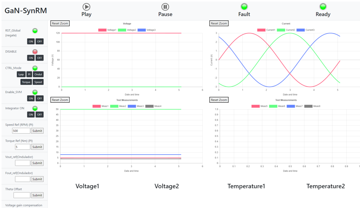
Fig. 5.9. Webpage produced by the SoC for graphical user interface.
