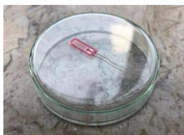
Figura 5-26 – *Strain Gauge* (*sg*)
