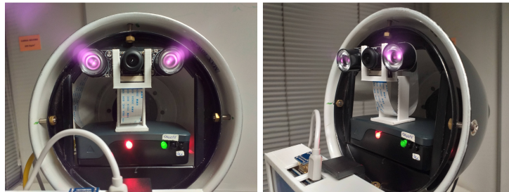
Figure 4.4: The inside of the lampshade of the chosen light fixture, in which the prototype was encased. A metal support was built and screwed to the inside of the lampshade, to accommodate the RPI and keep it and the camera level.
