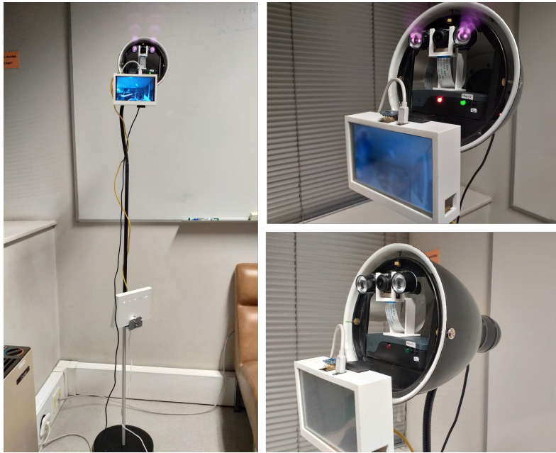
Figure 4.6: The final build of the prototype for Lampsy. The RPI was placed inside its official case and buttons and LEDs were installed in it. A support for the camera was 3D printed and glued to the case. This was then placed inside a floor lamp, to which a display was attached, inside a custom 3D printed encasing.
