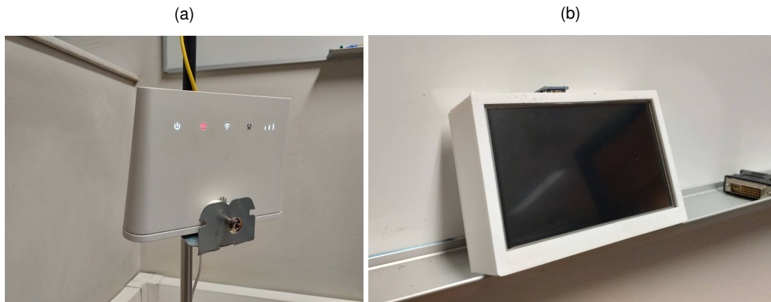
Figure B.3: (a) – The support built for the 4G router, attached to the lamp pole, with the router placed on it. (b) – The 3D model for the display encasing, designed with the 3D modelling software OpenSCAD and 3D printed using the BEETHEFIRST+ 3D printer located at IT.
