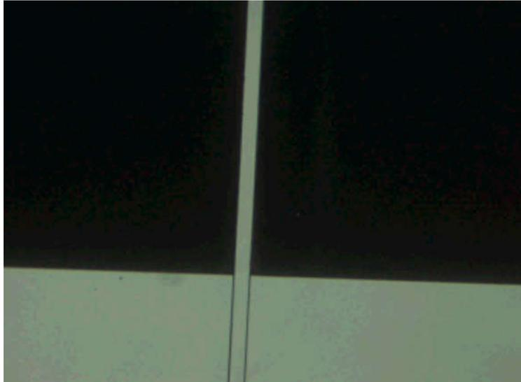
Figure 7.2 - Image obtained by microscopy of the microfluidic platform with aluminum electrodes. The micrograph was obtained where the microchannel meets the aluminum electrodes and after the etching of the gap. The microchannel has a width of 50  $\mu\text{m}$ , a height of 20  $\mu\text{m}$  and a length of 3 cm. The black portion is the opaque aluminum.
