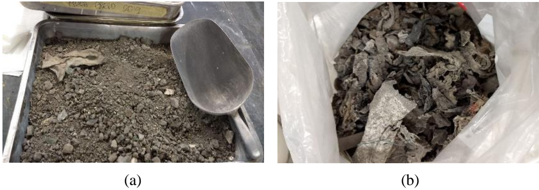
Figure 3 - Dry MIBA (a) and contaminants removed by manual cleaning (b)
