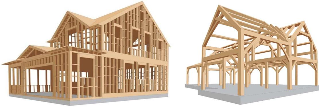
**Figure 1.** Examples of a light wood-frame (left) and a post-and-beam timber frame (right).
