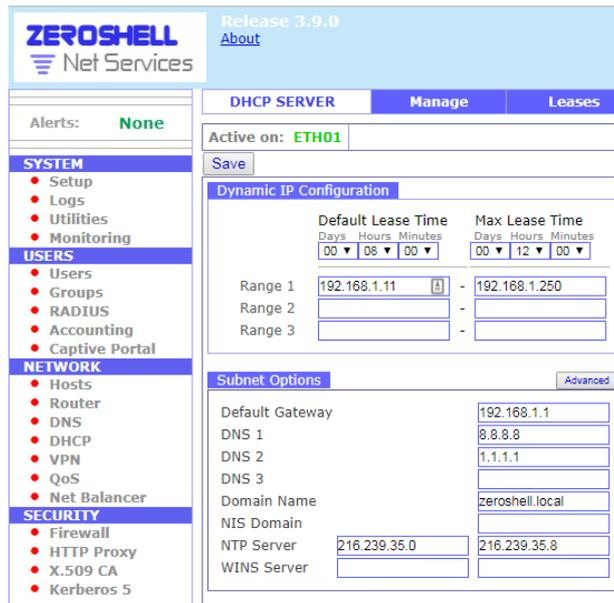
Figure 4.17: Zeroshell's Dynamic Host Configuration Protocol (DHCP) server configuration
