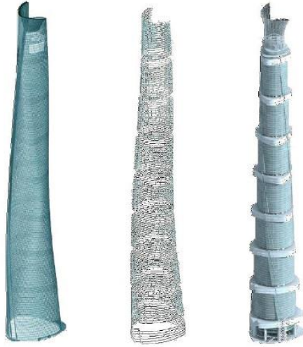
Figure 4.27 - Curtain Wall A, CWSS and Curtain Wall B (left to right) (Nichols, 2014)
