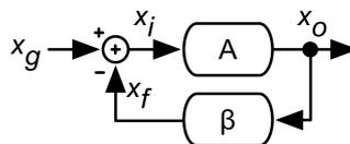
Figure 2-16. Generic system with feedback.
