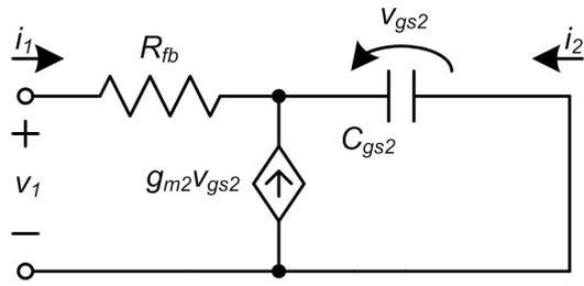
Figure A-11. Feedback block:  $v_2 = 0V$ .
