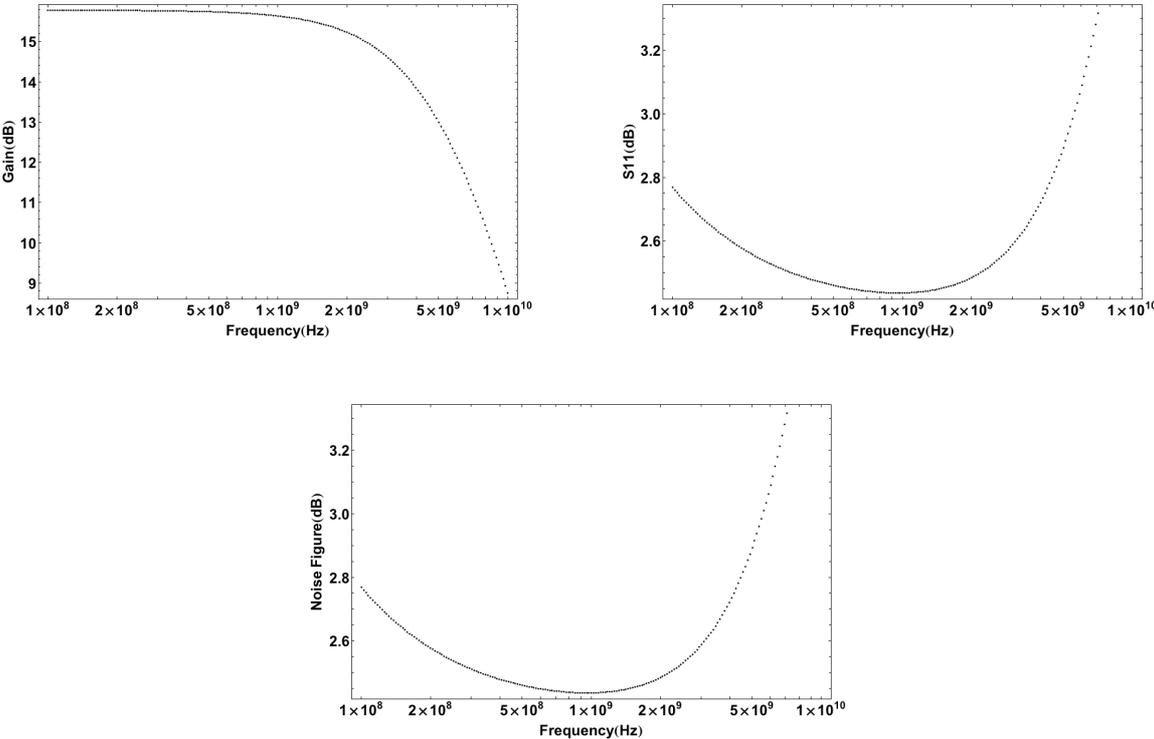
Figure A-17. Gain, S<sub>11</sub> and NF plots of LNA\_A.
