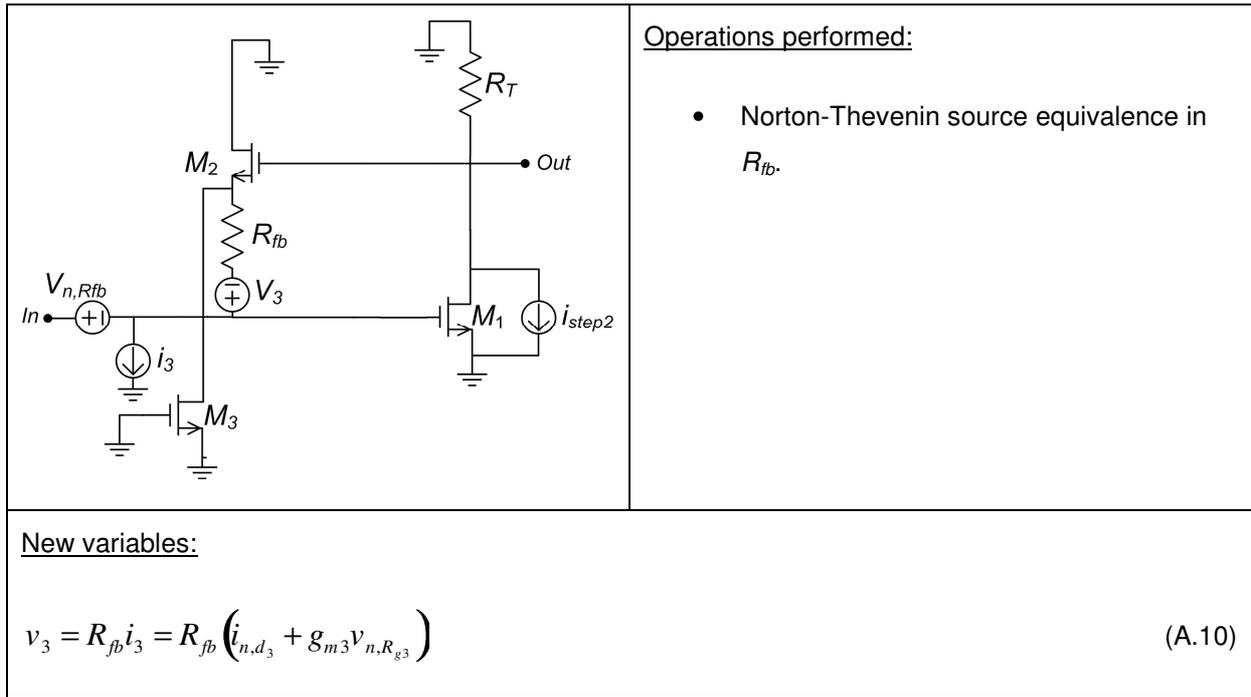
Step 3 of the noise source transformations for LNA\_A.
