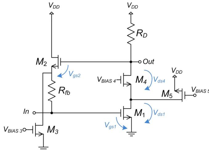
Figure 4-6. Critical path for the LNA\_A.
