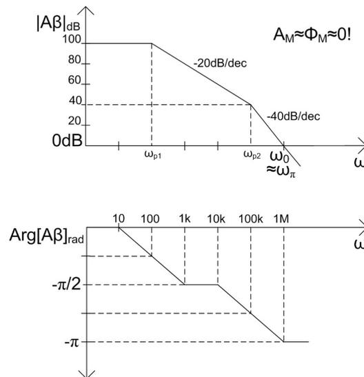
Figure 2-21. Example of asymptotic Bode diagrams for loop gain with two poles.
