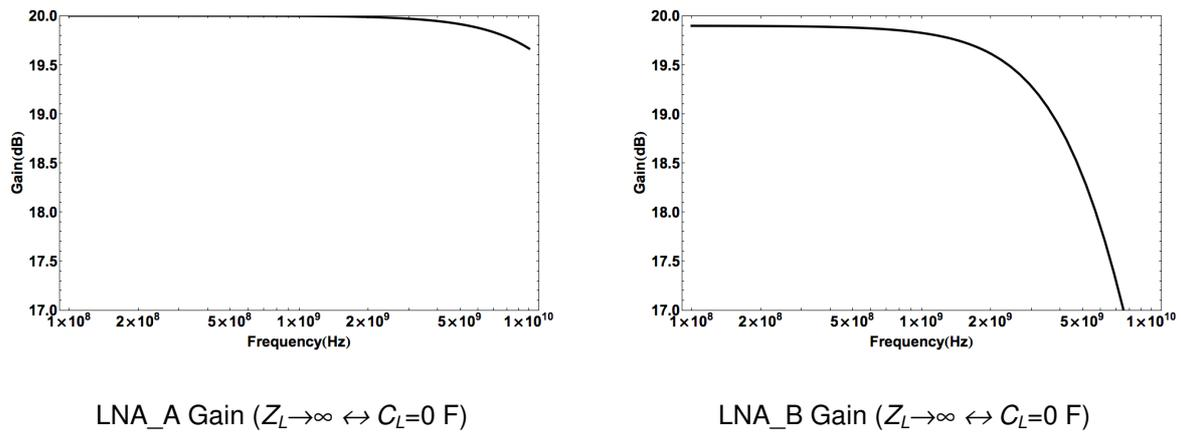
Figure 4-8. Gain of LNA\_A and LNA\_B with infinite load impedance.
