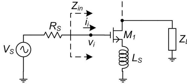
Figure 3-4. Common-Source LNA with inductive degeneration (biasing not represented).
