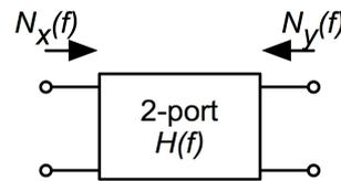
Figure 2-11. 2-port with transfer function  $H(f)$  excited by noise source with power density  $N_x(f)$ .
