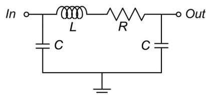
Figure 6-5. Bonding wire model.
