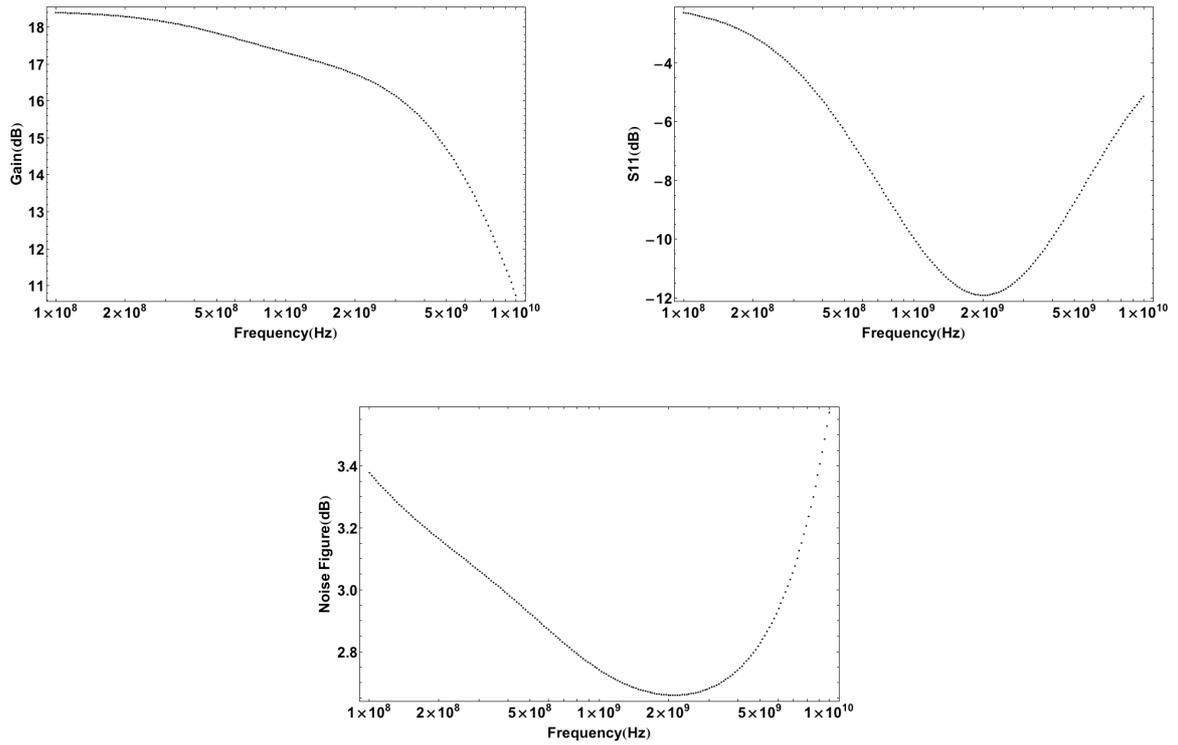
Figure A-19. Gain,  $S_{11}$  and NF plots of LNA\_B.
