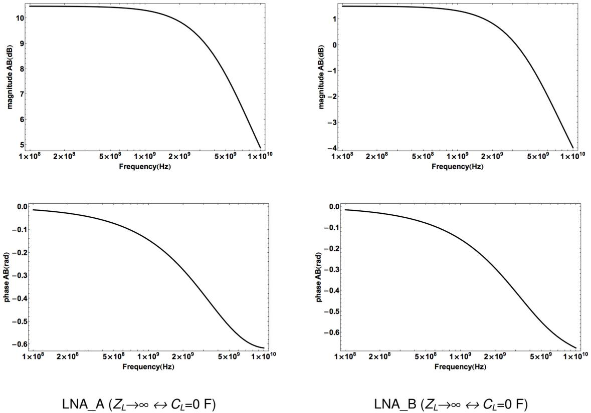
Figure 4-13.  $|A'\beta_{ideal}|$  and  $\phi(A'\beta_{ideal})$  of LNA\_A and LNA\_B with infinite load impedance.
