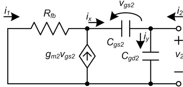
Figure A-10. Feedback block:  $v_1 = 0V$ .
