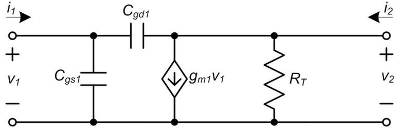
Figure 4-4. Small signal circuit of the amplifying block.
