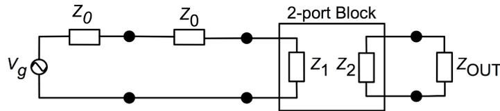
Figure 2-6. 2-port block connected to a transmission line and  $Z_{OUT}$ .
