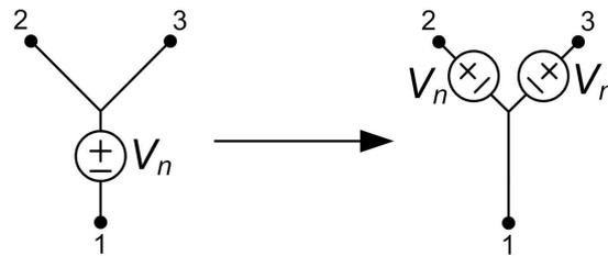
Figure A-2. Voltage source shifting.
