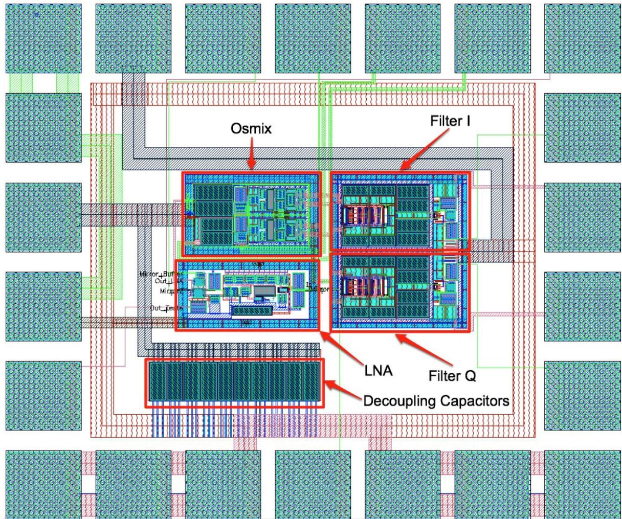
Figure 6-11. Layout of the radio receiver.
