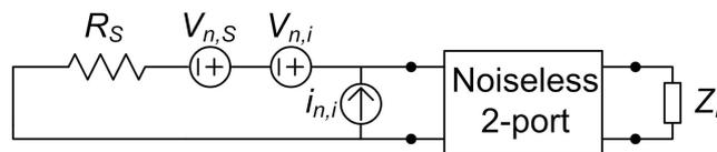
Figure 2-13. Noisy 2-port excited by signal and noise source.
