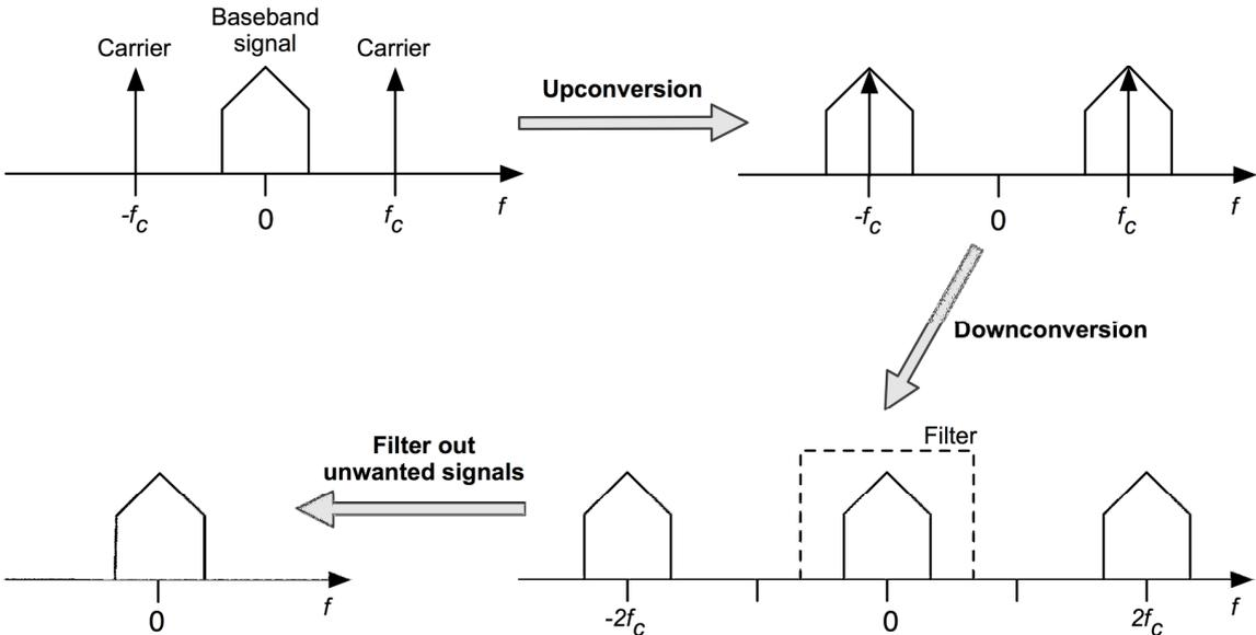
Figure 2-2. Upconversion and downconversion exemplified (homodyne system).
