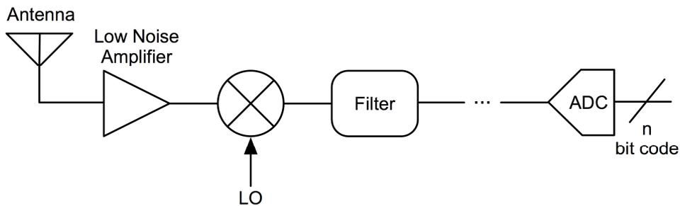
Figure 2-4. Block diagram of a wireless receiver.
