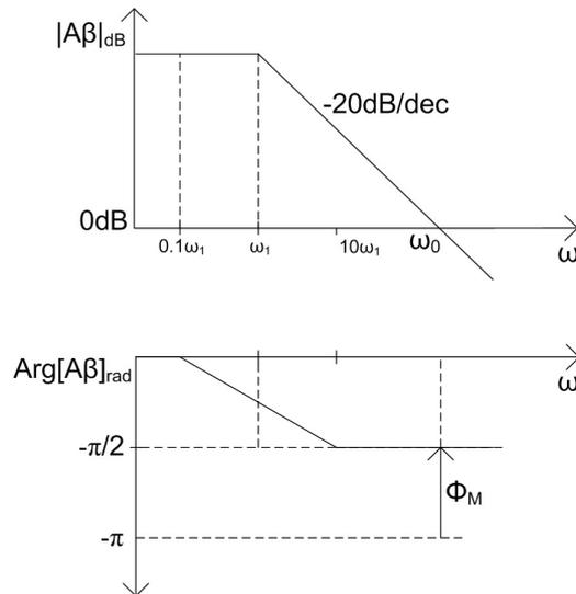
Figure 2-20. Asymptotic Bode diagrams for loop gain with only one pole.
