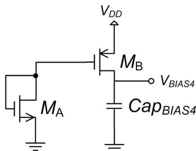
Figure 6-4.  $M_4$  Pull-up circuit.
