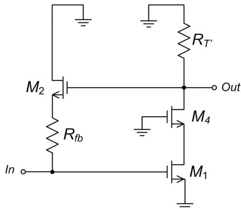
Figure 4-3. Small signal circuit of LNA\_A and LNA\_B.
