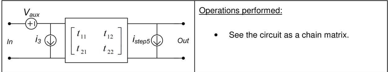
Step 6 of the noise source transformations for LNA\_A.
