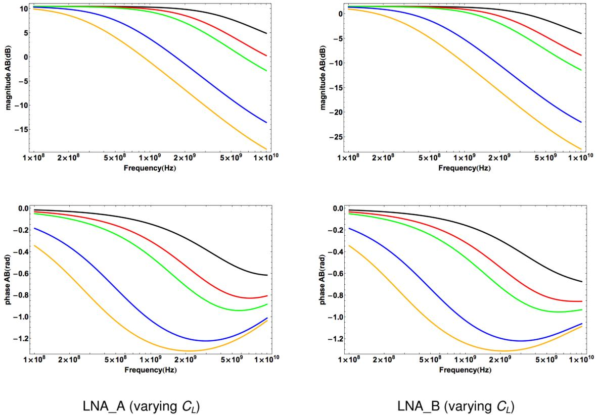
Figure 4-14.  $|A'\beta_{ideal}|$  and  $\phi(A'\beta_{ideal})$  of LNA\_A and LNA\_B for different values of output capacitance.  $C_L=0$  F (Black) ;  $C_L=50$  fF (Red) ;  $C_L=100$  fF (Green) ;  $C_L=500$  fF (Blue) ;  $C_L=1$  pF (Orange).
