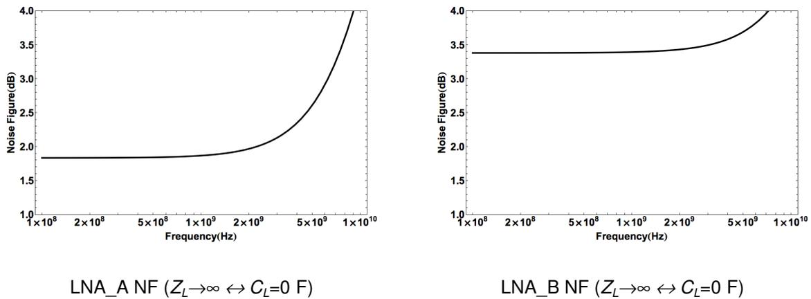
Figure 4-12. Noise Figure of LNA\_A and LNA\_B with infinite load impedance.
