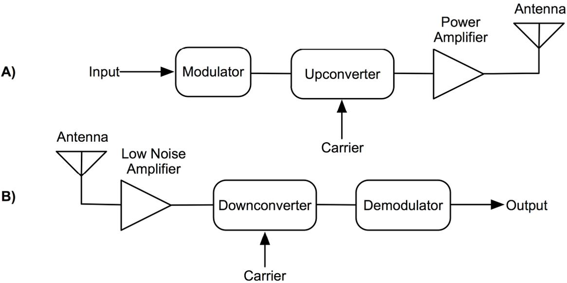
Figure 2-1. Block diagram of a generic analog RF system: A) Transmitter B) Receiver.
