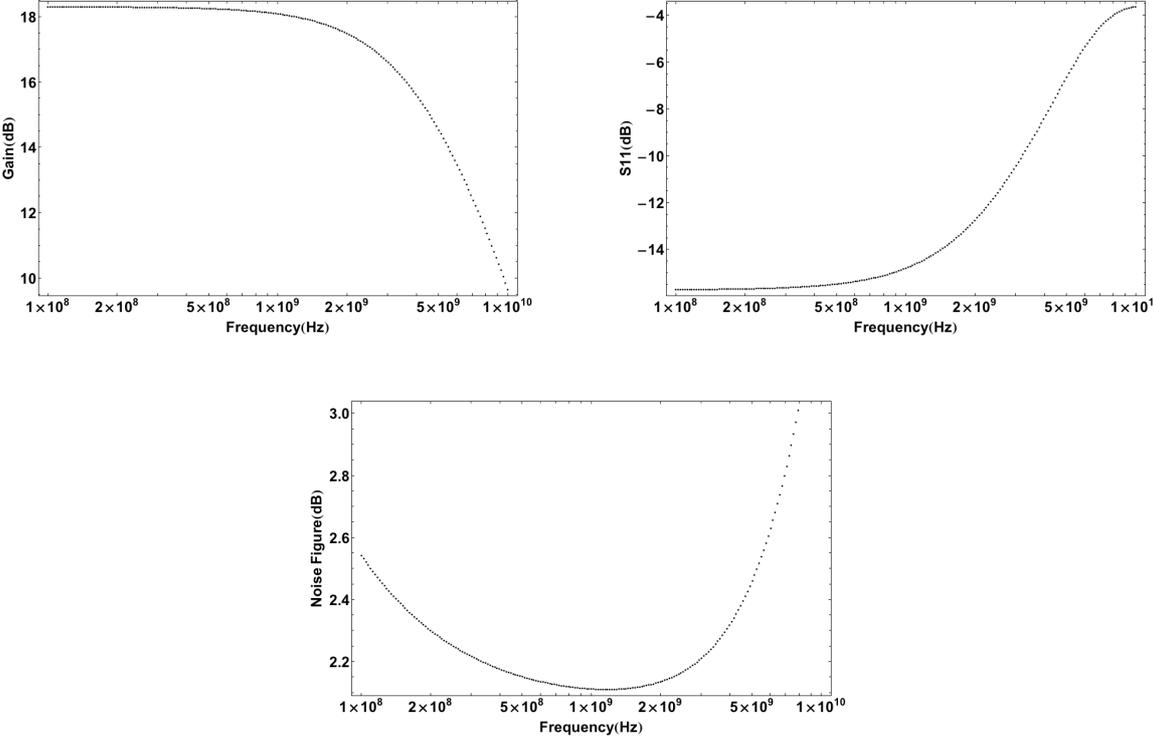
Figure A-18. Gain, S<sub>11</sub> and NF plots of MOSFET only LNA\_A.
