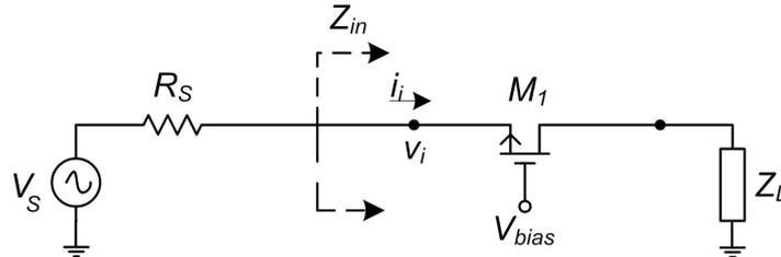
Figure 3-3. Common-gate LNA (biasing not represented).
