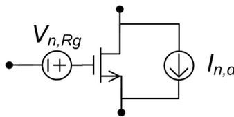
Figure 2-15. MOS transistor noise sources for RF design.
