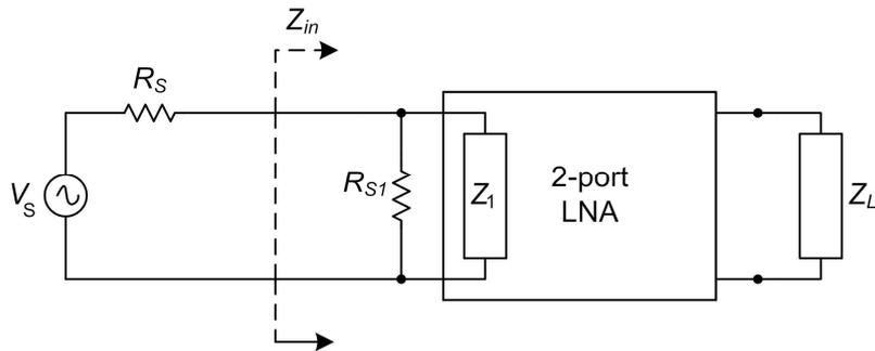
Figure 3-2. LNA using Input Resistor.
