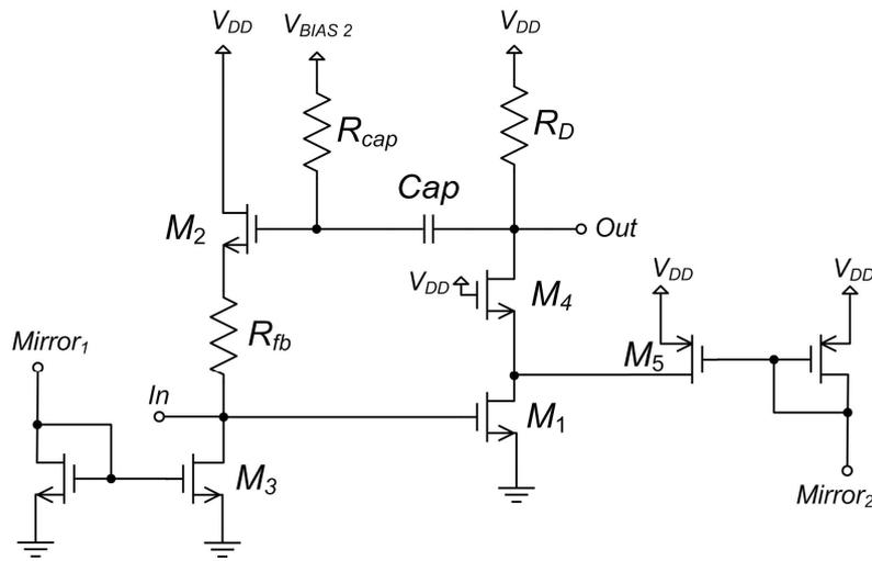
Figure 5-3. Schematic of the simulated LNA\_B.
