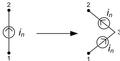
Figure A-3. Splitting of a noise source.
