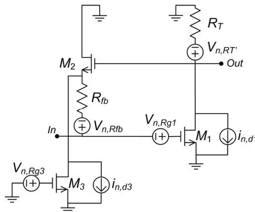
Figure A-15. LNA\_A and its relevant noise sources.
