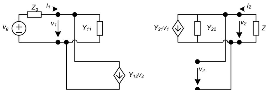
Figure 2-18. Transresistance amplifier rearranged.
