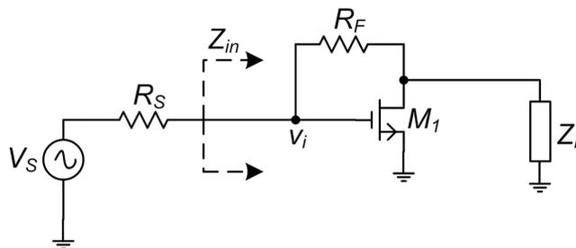
Figure 3-5. LNA with resistive feedback (biasing not represented).
