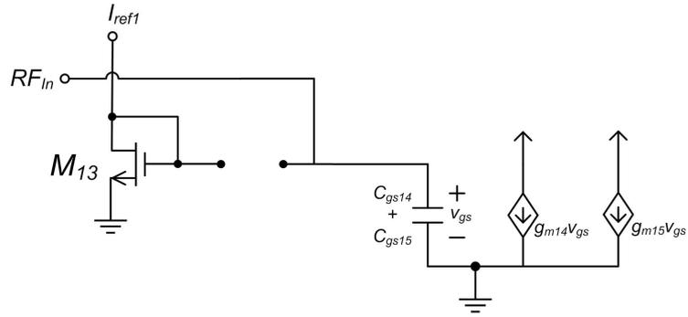
Figure A-14. Small-signal circuit of the input of the OSMIX block.
