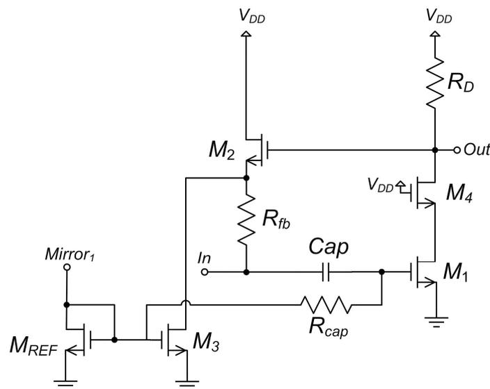
Figure 5-4. Schematic of the simulated LNA\_C.
