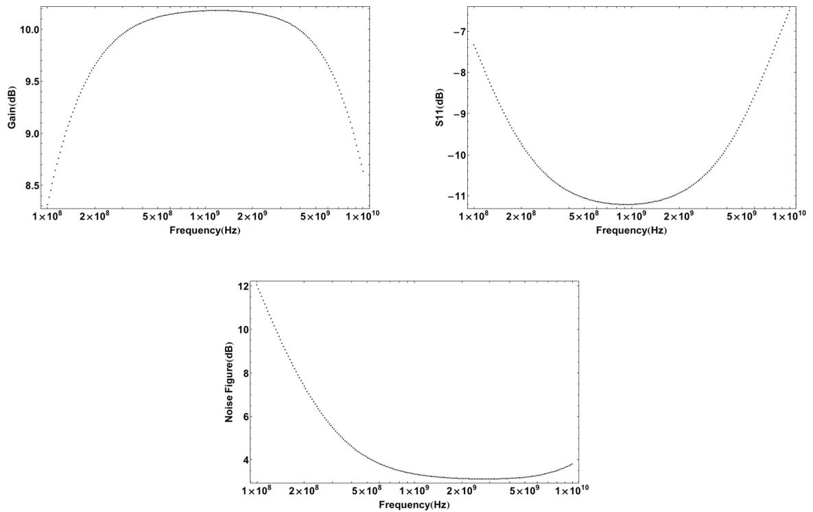
Figure A-20. Gain,  $S_{11}$  and NF plots of LNA\_C.
