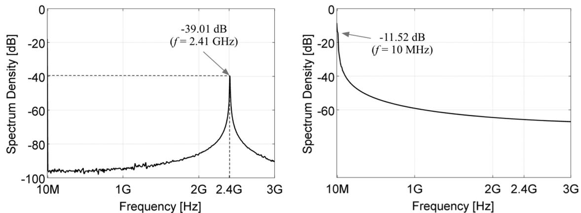
Figure 6-9. Radio receiver input/output plot of a signal discrete Fourier transformation.
