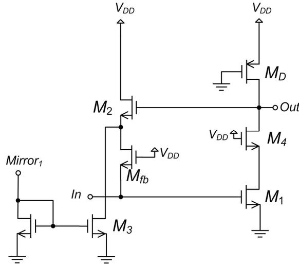
Figure 5-2. Schematic of the simulated MOSFET only LNA\_A.
