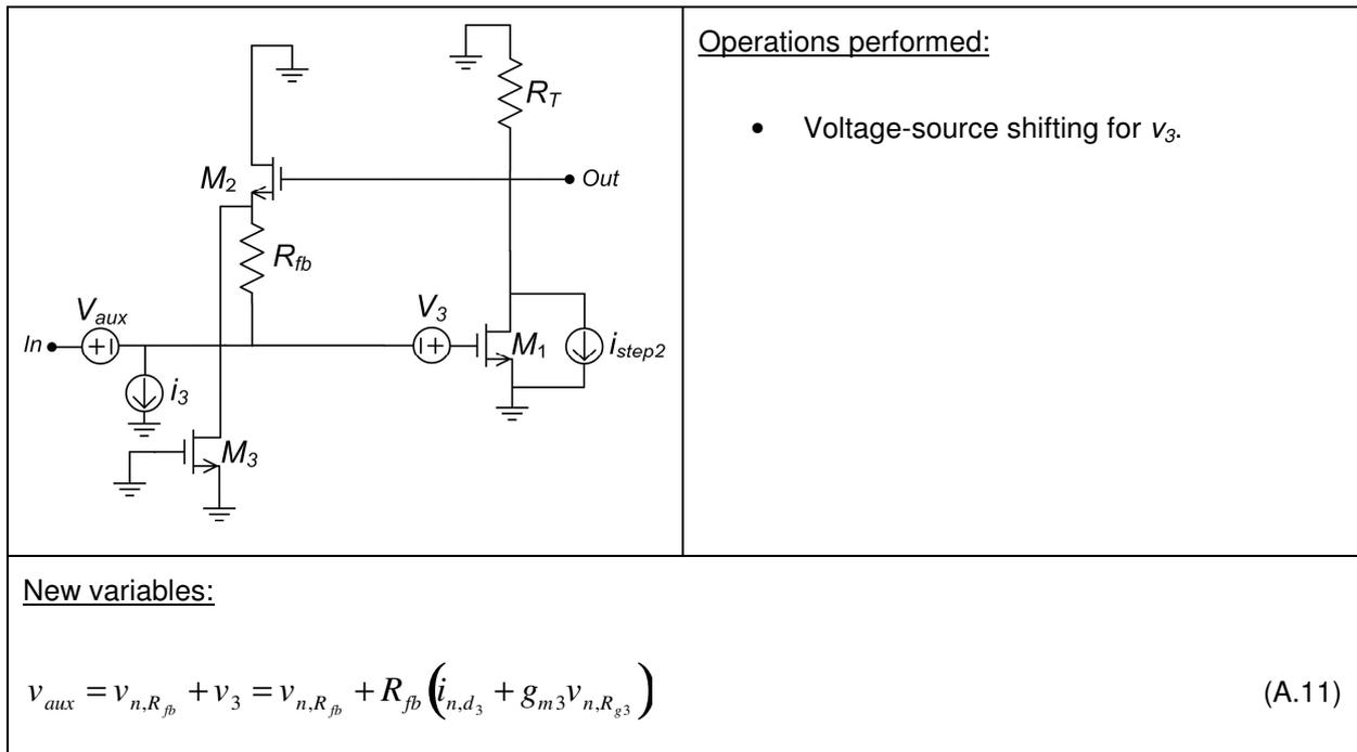
Step 4 of the noise source transformations for LNA\_A.
