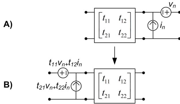
Figure A-5. 2-port transformation of noise sources.
