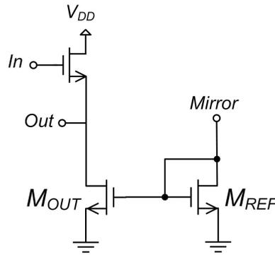
Figure 6-1. Buffer schematic.
