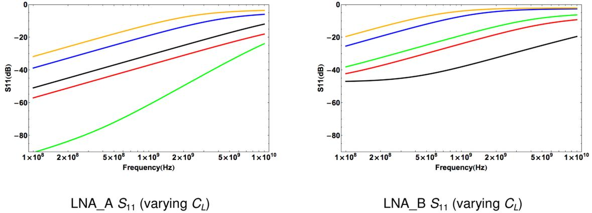
Figure 4-11.  $S_{11}$  of LNA\_A and LNA\_B for different values of load capacitance.  $C_L=0$  F (Black);  $C_L=50$  fF (Red);  $C_L=100$  fF (Green);  $C_L=500$  fF (Blue);  $C_L=1$  pF (Orange).
