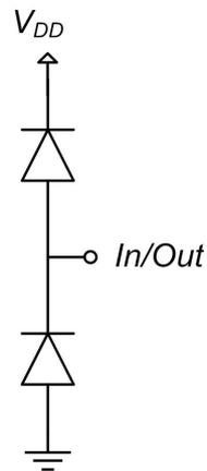
Figure 6-3. ESD protection diodes.
