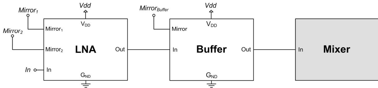
Figure 6-2. LNA, buffer and mixer connections.
