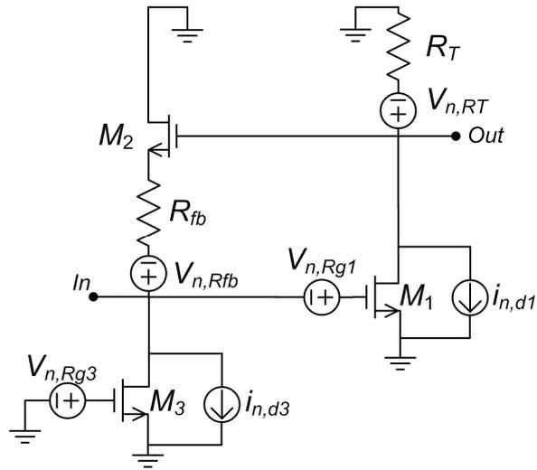
Figure A-16. LNA\_B and its relevant noise sources.
