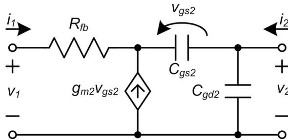
Figure 4-5. Small signal circuit of the feedback block.
