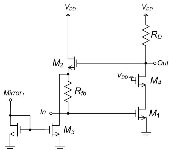
Figure 5-1. Schematic of the simulated LNA\_A.
