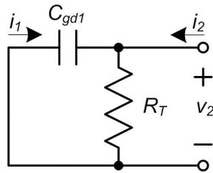
Figure A-7. Amplifying block:  $v_1 = 0V$ .
