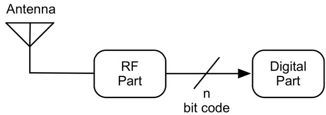
Figure 2-3. Possible block diagram of a wireless receiver.
