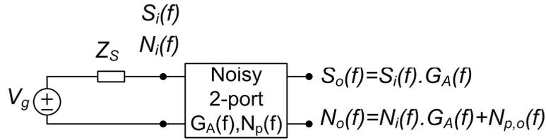
Figure 2-12. Noisy 2-port excited by signal and noise source.
