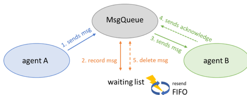
Figure 4.18 - Message scheme to reproduce FIFO function.
