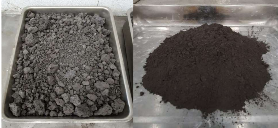
2 Figure 3: EAFS as-received (a- left) and after milling to the required size for use as a precursor in concrete (b-right)
