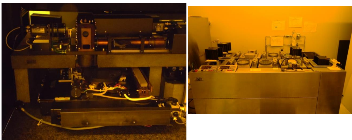
Figure 29 – Photographs taken in the yellow room: a) DWL stage and laser system; b) coating and development tracks on the SVG track system.
