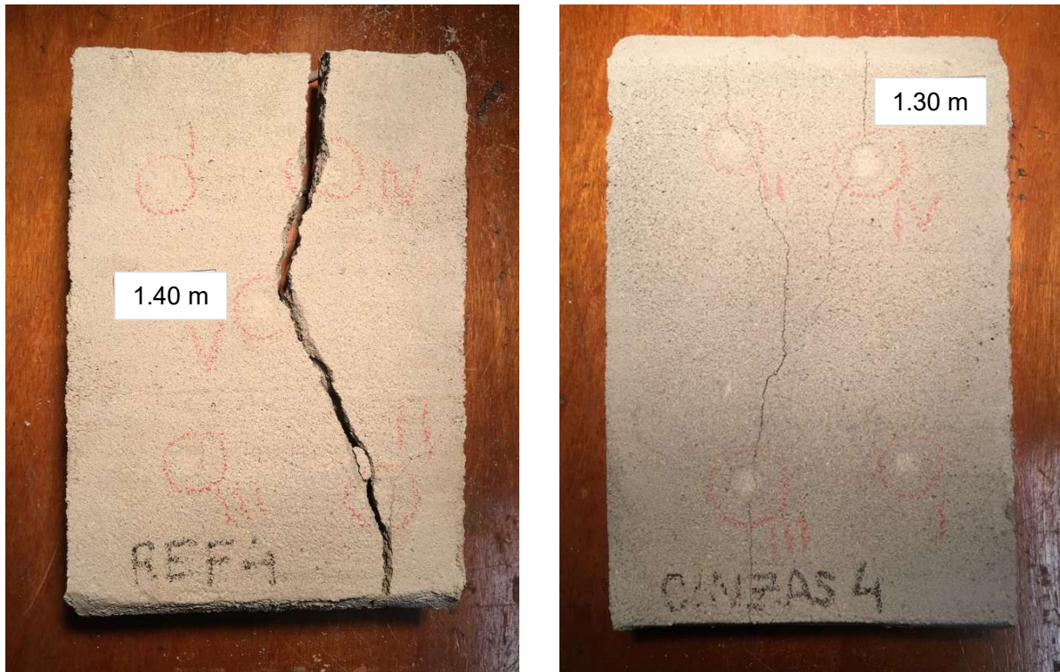
Figure 9. Resistance to impact (failure) - REF (left) mortar and FBA (right) mortar
