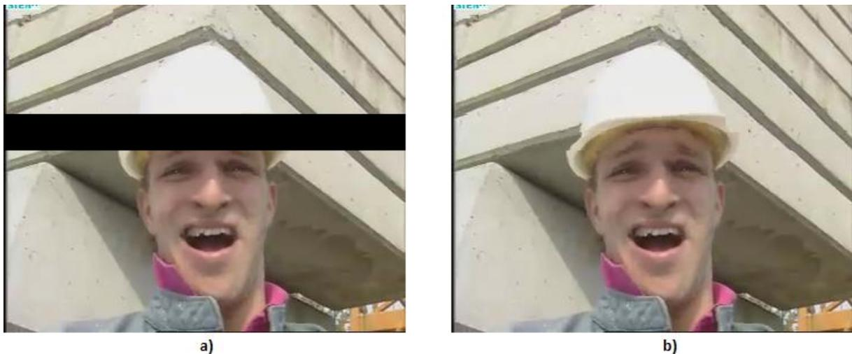
Figure 48 - Successful error concealment a) where the loss occurred b) decoder output
