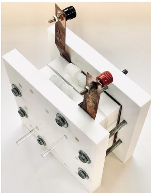
**Figure 4.2:** Fully assembled VRFB cell.
