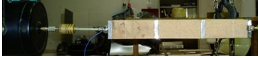
Figure 4.25 – Photograph of the experimental test prototype periodic bar with square cross-section with a side length of 0.050m, composed of 3.5 unit cells, i.e., four steel and three CCM ref. 8123 half-cells each with a length of L_{Mat_1}=0.010\text{m} and L_{Mat_2}=0.100\text{m} , respectively. The half-cells are bonded with a structural adhesive creating a prototype with a total length of 0.340m [44].
