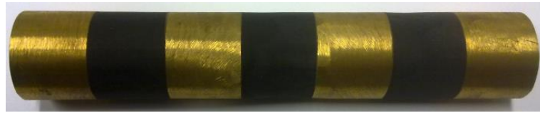
Figure 1.1 – 1D two-material phononic-inspired device for longitudinal vibration attenuation.
