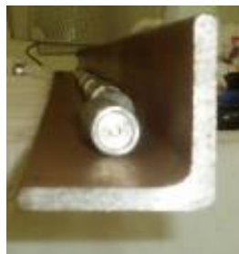
Figure A.5.2 – L shaped beam (side view) used to aid the centering of the cells during the cure of the adhesive.
