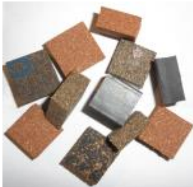
Figure A.5.1 – Steel and CCM layers.
