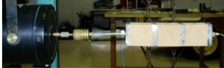
Figure 4.23 – Photograph of the experimental test prototype periodic bar with square cross-section with a side length of 0.050m, composed of 3.5 unit cells, i.e., four steel and three CCM (ref. 8123) half-cells each with a length of L_{Mat_1}=0.010\text{m} and L_{Mat_2}=0.050\text{m} , respectively [44].
