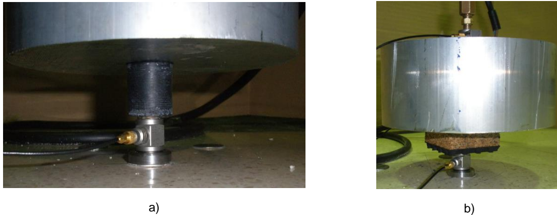
Figure 4.27 – Photograph of the experimental setup used to test the commercial vibration isolators: a) rubber mount (CVI-1); b) neoprene waffle and cork sandwich (CVI-2).
