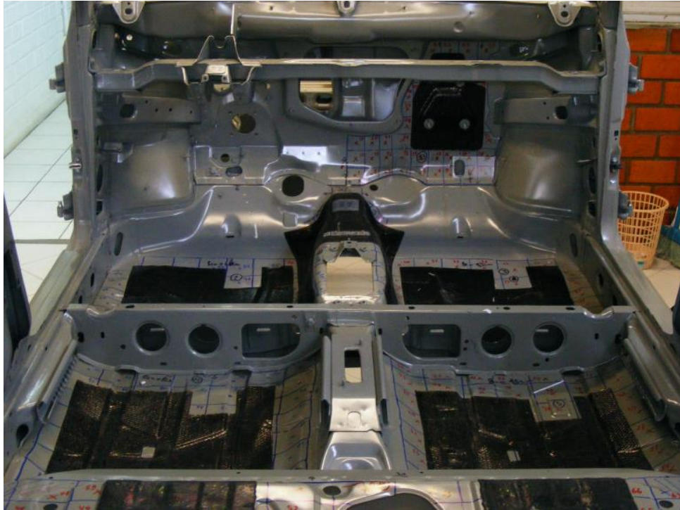
Figure 1.9 – Interior view of the front of an automobile with an FLD SDT applied. (Image reproduced from [70]).
