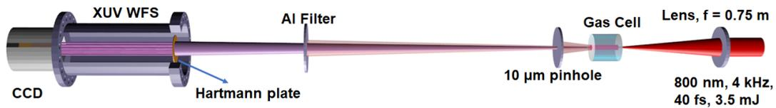
Figure 3.6: Schematic of the setup for calibration of XUV wavefront sensor
