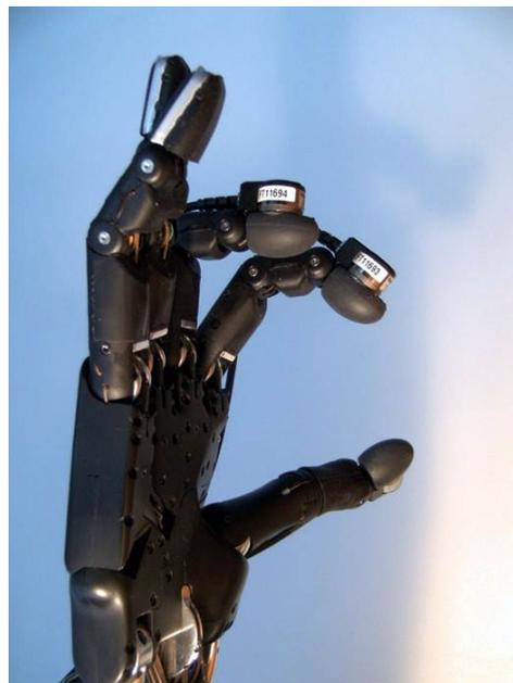
**Figure 1.1:** The Shadow Robot Hand equipped with fingertip force/torque sensors ATI NANO 17.
