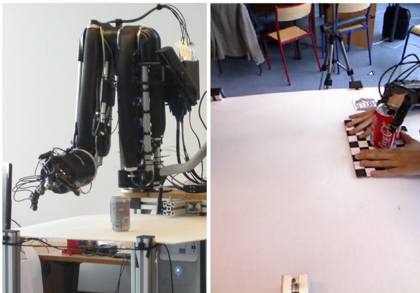
**Figure 4.28:** Shadow arm and hand that serves as main platform for the HANDLE project (left), image captured by the Kinect mounted on the arm during the course of the experiment.
