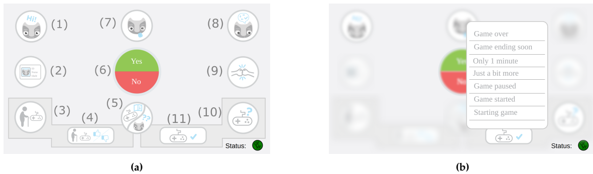
Figure 7.2: The dialogue control GUI (a) is composed by a set of buttons grouping several verbal intentions into categories. When pressed, the buttons will expand (b) presenting the available verbal intentions. Button icons were designed by Hugo Simão.
