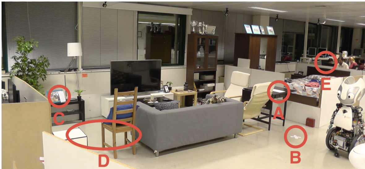
Figure 8.1: Setup of the user study. A - Task instructions; B - Initial Position; C - Target picture with geometric shapes; D - Two obstacles for the robot, a box and a chair; E - Researcher controlling the robot
