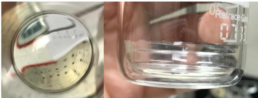
Figure 23: Thin PVA hydrogels: up and side views.
