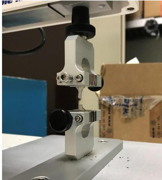
*Figure 17: Test set-up for tensile testing.*
