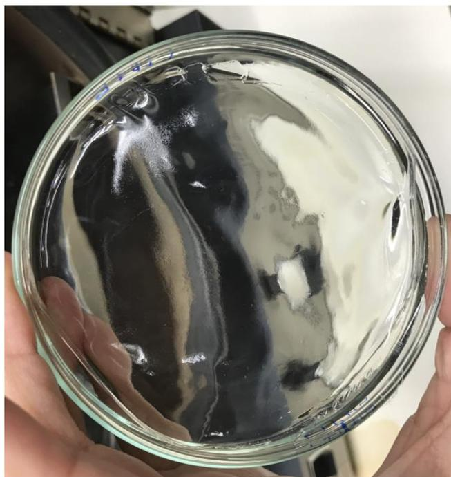
*Figure 24: Thick PVA hydrogel.*
