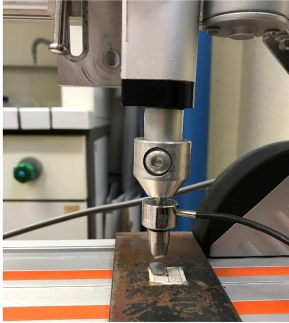
*Figure 18: Test set-up for compressive testing.*
