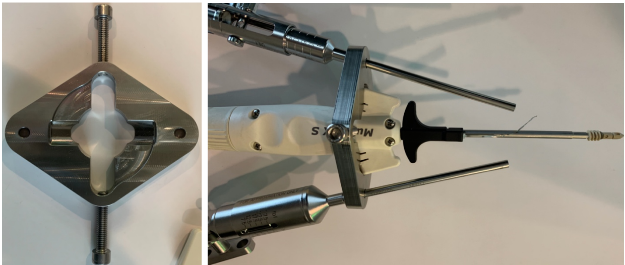
Figure 6.2 –Prototype (left); prototype, anchor and tensioners assembled (right).
