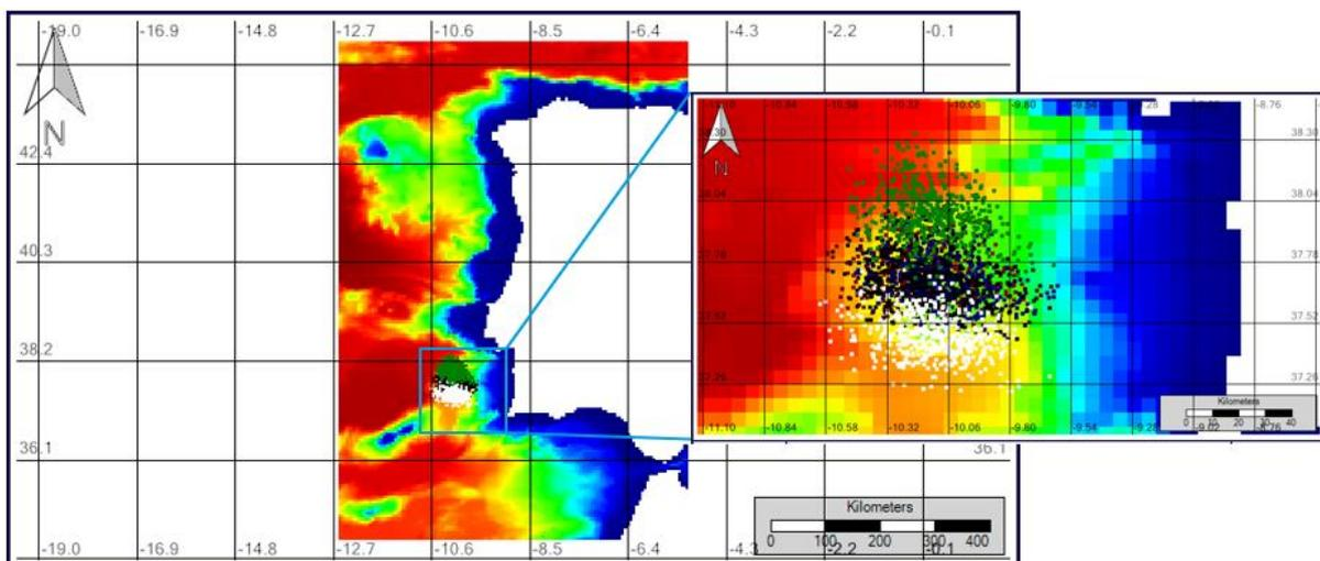
FIGURE 68 – OIL SICK LOCATION FOR WIND FORCING ANALYSIS ON THE 18<sup>TH</sup> JULY (BROWN – REFERENCE RUN; DARK BLUE – WINDX +20; BLACK – WINDX -20; WHITE – WINDY +20; RED – WINDY -20)
