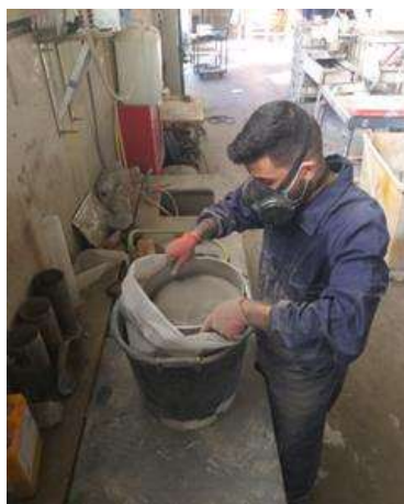
Figure 9 - MIBA sieving with 1 mm sieve (a); Container for preventing the humidity of MIBA (b)
