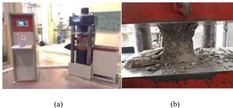
Figure 17 - Press machine (a) and sample reaching failure load (b)
