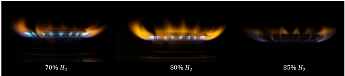
Figure 4.2: Flames Appearance without Pan - B10 1500W
